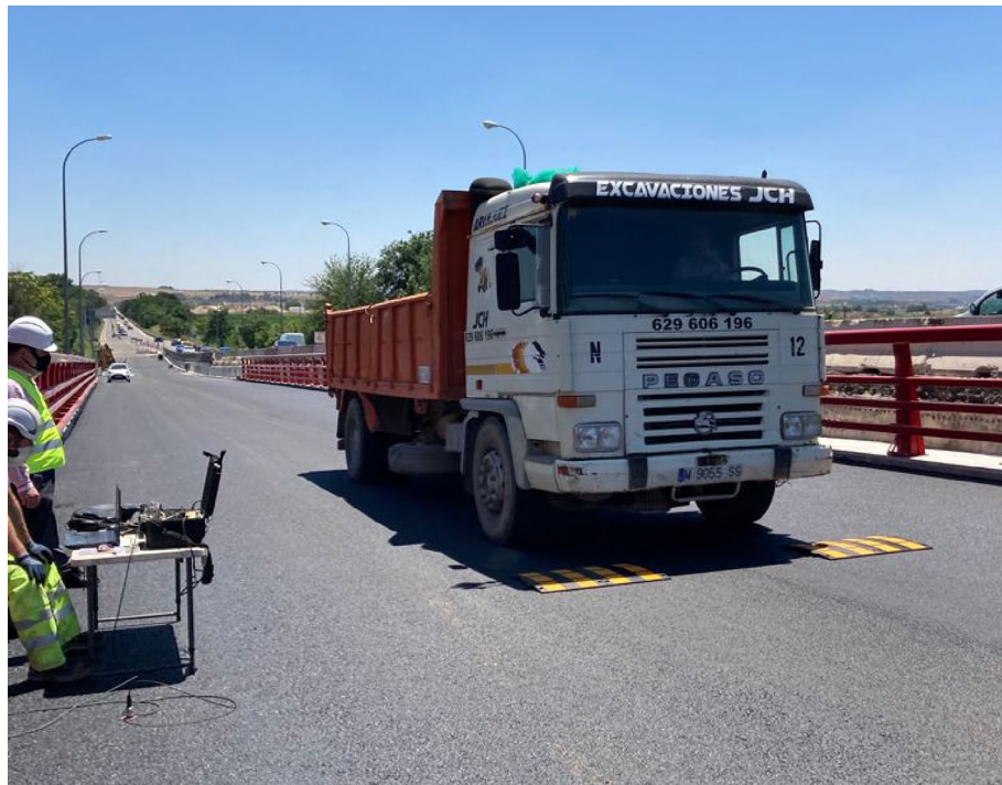
Figure 10. Truck passing over Rilem plate.
