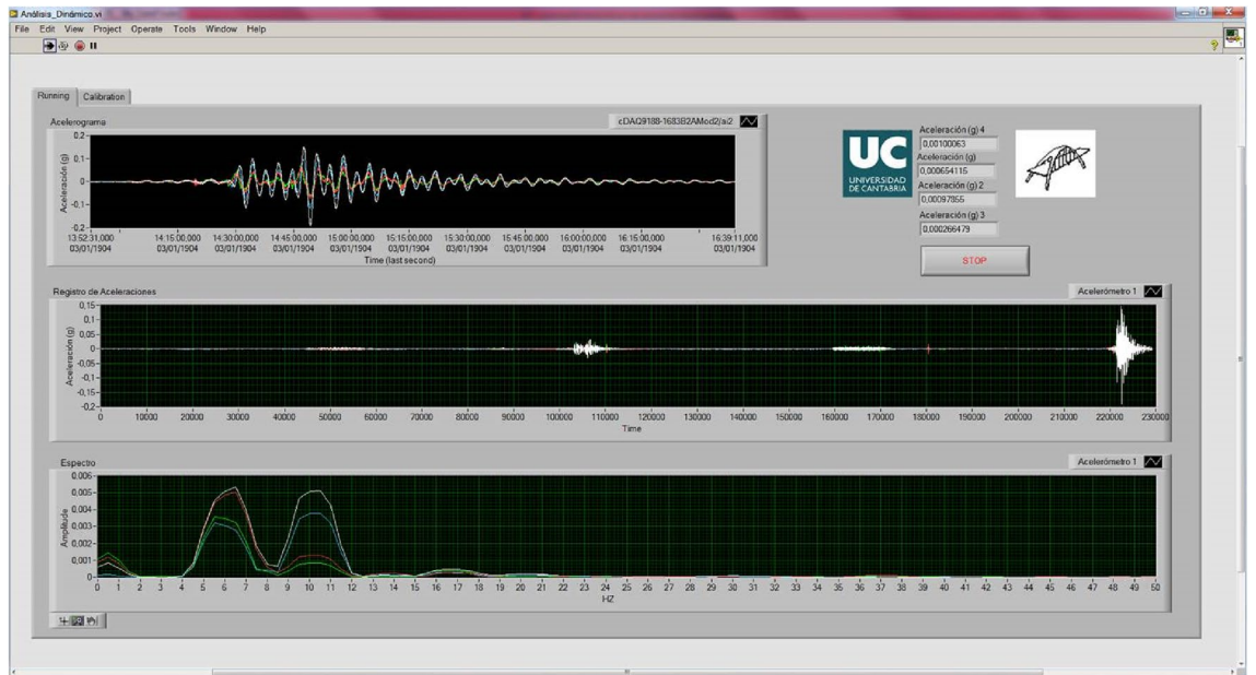
Figure 12. Real-time visualization of the data provided by the accelerometers.
