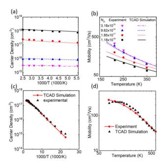
FIGURE 3. Comparison of experimental [18], [20] and TCAD PhuMob electron mobility and free carrier concentration data in Si-doped ((a)-(b)) and Ge-doped ((c)-(d)) Ga<sub>2</sub>O<sub>3</sub>.
