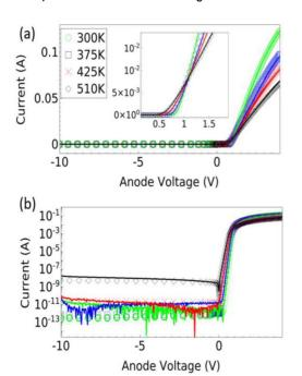
FIGURE 5. Experimental (lines) and TCAD simulated (markers) I-V curves in (a) linear and (b) log scale at different temperatures. Inset shows the I-V curves in the turn-on region.
