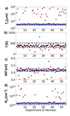
FIGURE 11. Prediction of experimental device parameters with (black) and without (red) PCA. Blue dash lines show the expected boundaries of the parameters based on physical analysis. Some red markers (without PCA) cannot be shown because they are outside of the plotting ranges. Each experimental IV from Fig. 10 is represented on the x-axes.
