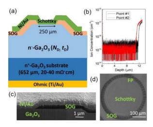
FIGURE 2. (a) Schematic of the fabricated vertical Ga<sub>2</sub>O<sub>3</sub> power Schottky barrier diodes; (b) An exemplary illustration of the drift layer thickness at two spots on the wafer determined by the Si profile measured by secondary ion mass spectrometry. (c) Cross-sectional scanning electron microscopy (SEM) image of the field plate region; (d) Top-view SEM image of the fabricated device.
