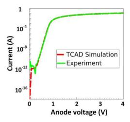
FIGURE 9. Experimental I-V curve and calibrated TCAD I-V curve showing big difference at V < 0.4 V due to measurement equipment limitation, despite very good overall calibration.
