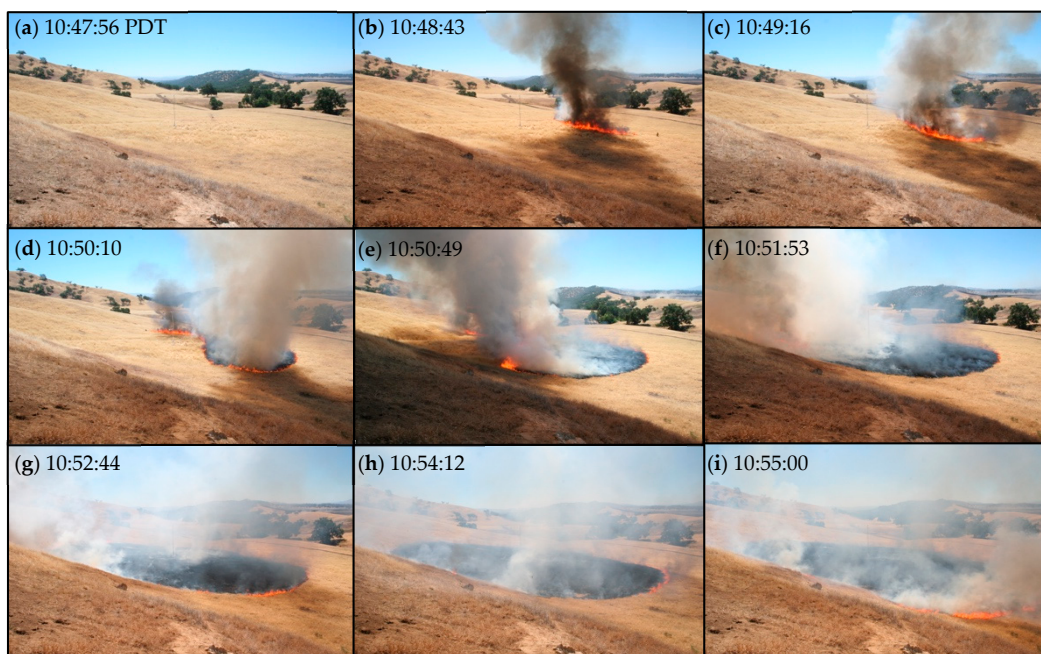
Figure 8. (a–i) Photographic time series showing fire front positions and plume structures, taken from a remote camera located in the burn unit (see Figure 2a). Times indicated are HH:MM:SS (PDT). Please refer to Figure 1 for plot orientation. Camera was located at location c in Figure 1.
