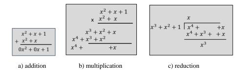
Figure 2. Examples of arithmetic in  $GF(2^3)$
