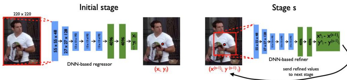
Figure 2. Left: schematic view of the DNN-based pose regression. We visualize the network layers with their corresponding dimensions, where convolutional layers are in blue, while fully connected ones are in green. We do not show the parameter free layers. Right: at stage s , a refining regressor is applied on a sub image to refine a prediction from the previous stage.
