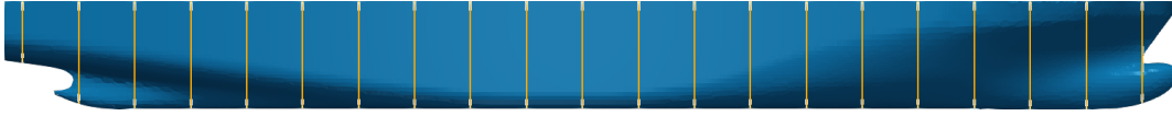
Figure 8.5: The surface of the DTC hull. The highlighted sections divide the ship into 20 equispaced chunks at the free-surface level.
