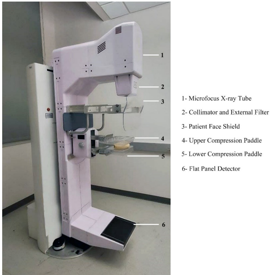
Figure 4.1: Phase Contrast Breast Tomosynthesis system (Hologic, Inc. MAN-05666, Revision 002, Marlborough, MA, U.S.A.)
