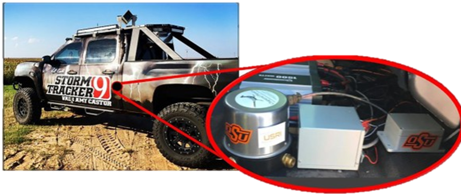
Figure 2.2: Image of GLINDA-housing storm chasing vehicle showing approximate location and configuration of install.
