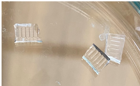
Figure 1: Representative fabricated PDMS stamps using penny columns as a mold.
