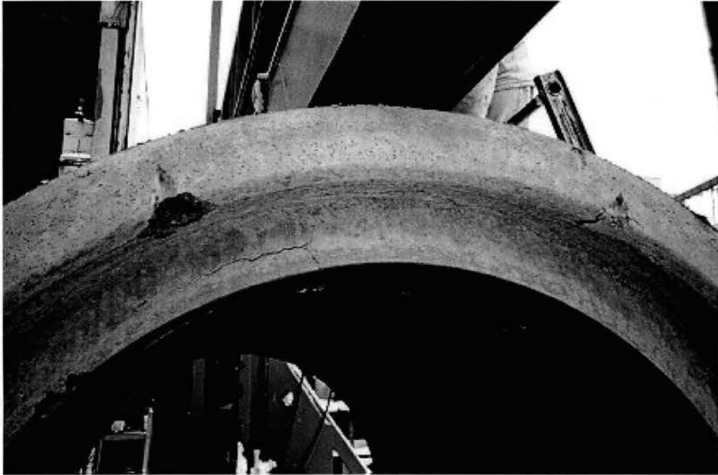
Figure B-27. Surface Crack Near Upper Load Point
