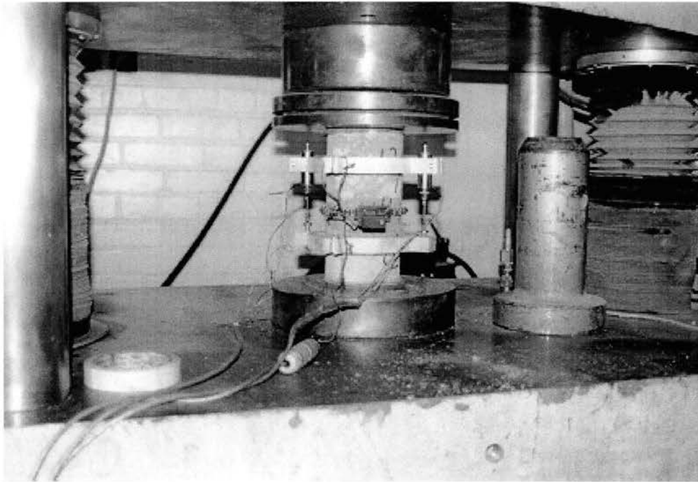
Figure B-3. Testing Machine Used for Static Modulus of Elasticity by ASTM C469
