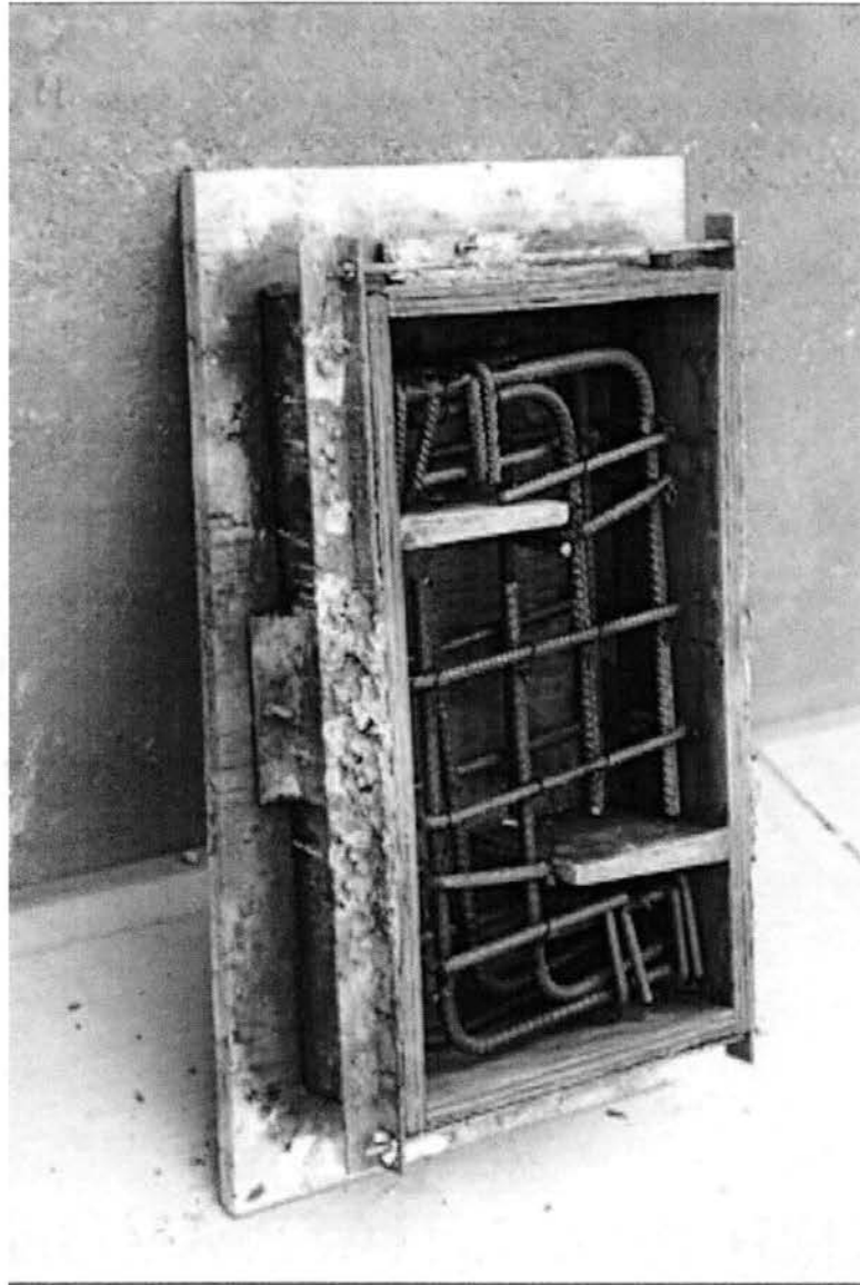
Figure 3-2. Push-Off Specimen Form
