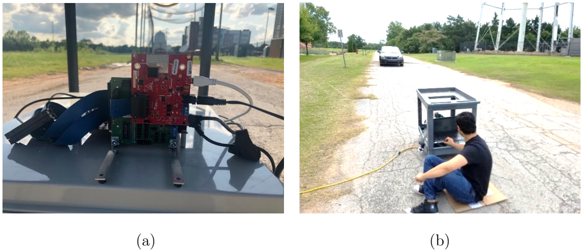
Figure 5.8: Measurement using TI radar (a) Radar used for the measurement (b) Experimental Setup
