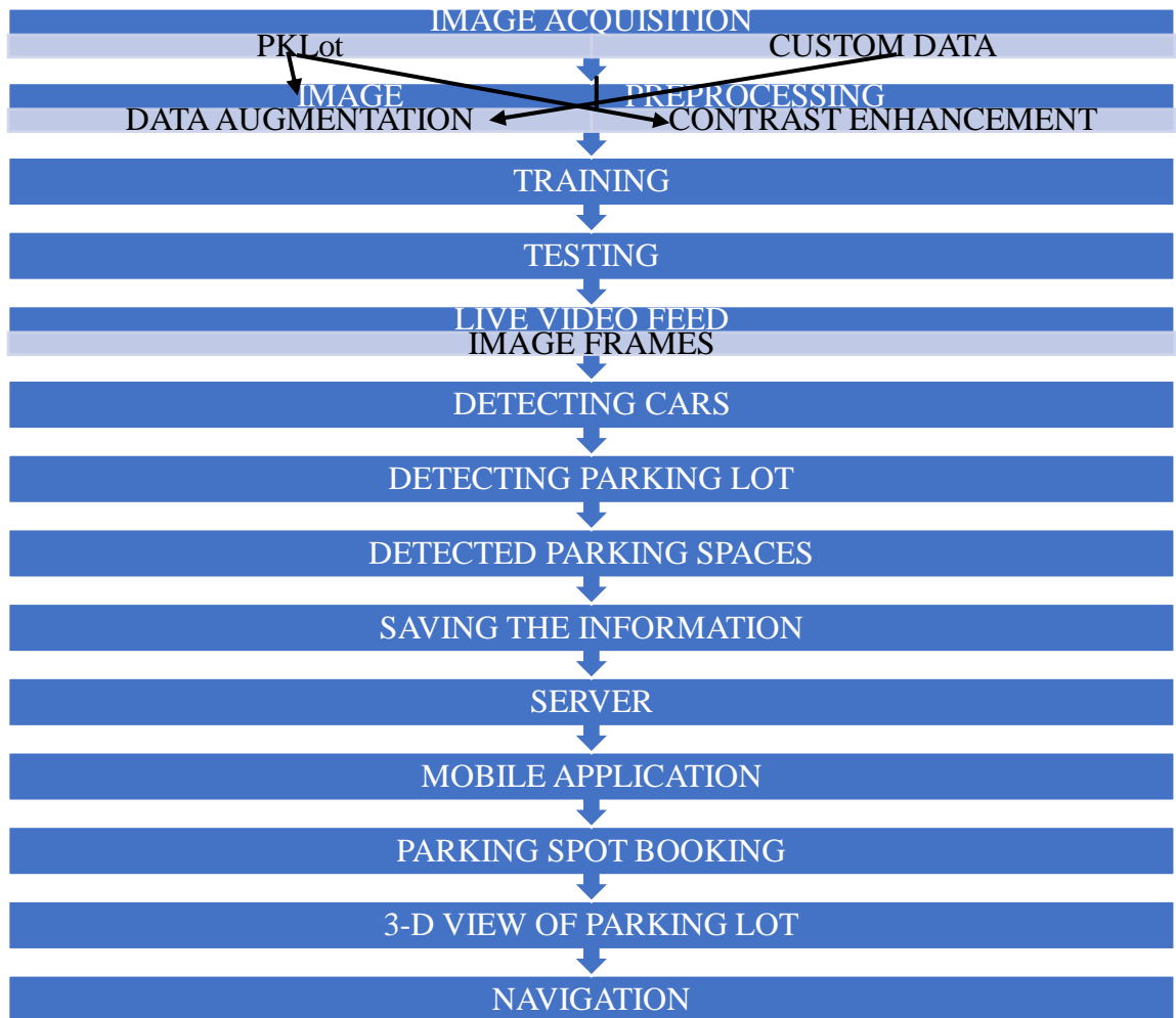
Figure 27 Flowchart of proposed Parking lot detection technique
