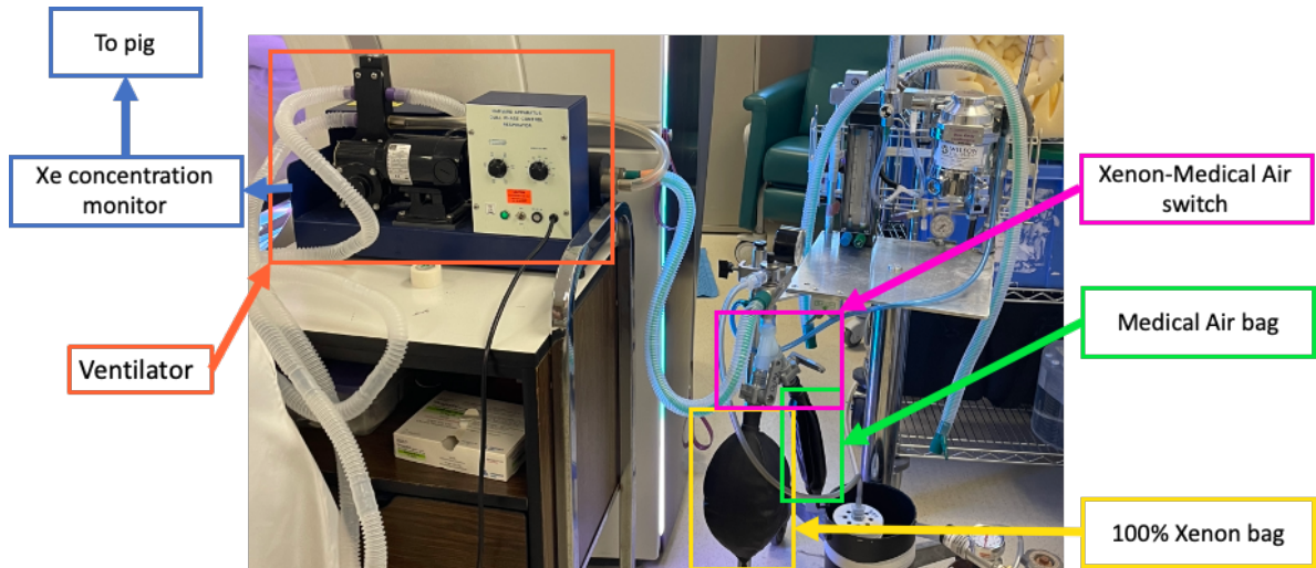
Figure 4-1 Experimental setup used for Xe-enhanced ventilation imaging.
