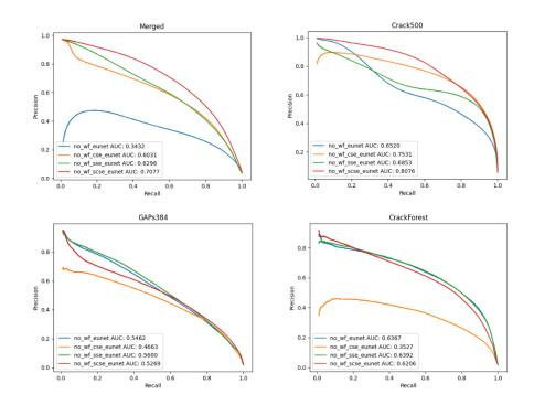
Figure 39: The Precision-Recall Curves (PRC) and corresponding AUPRC scores for the Efficient U-Net models without the atrous waterfall block
