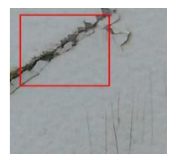
Figure 6: Crack detection result shown with bounding boxes [57]
