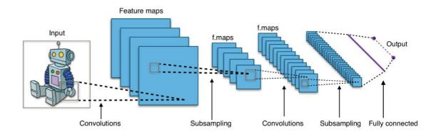
Figure 2: Convolutional Neural Network with Fully Connected Layers [85]
