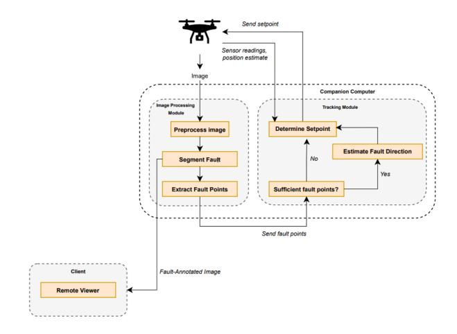
Figure 12: High-Level Proposed System Architecture
