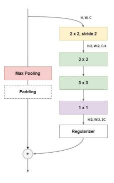
Figure 34: Encoder block in Efficient U-Net
