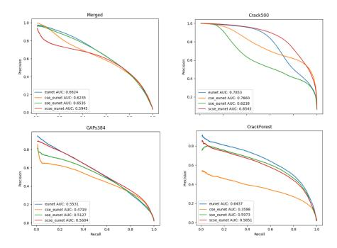
Figure 40: The Precision-Recall Curves (PRC) and corresponding AUPRC scores for the Efficient U-Net models with the atrous waterfall block
