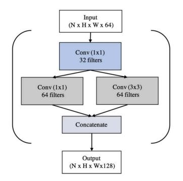
Figure 11: A fire module used in Squeeze U-Net [45]
