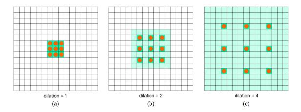
Figure 10:  $3 \times 3$  convolutions with different dilation rates: (a) - 1, (b) - 2, (c) - 4 [29]
