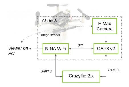
Figure 14: AI-deck system architecture [61]
