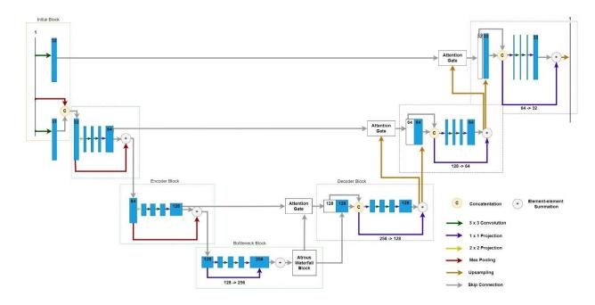
Figure 33: Proposed Efficient U-Net Architecture. Blue blocks represent feature maps, with the width denoting feature space and height denoting resolution
