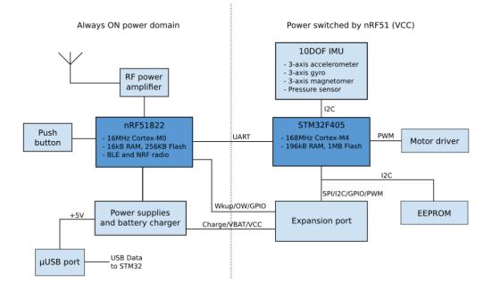
Figure 13: The Crazyflie 2.X system architecture [80]
