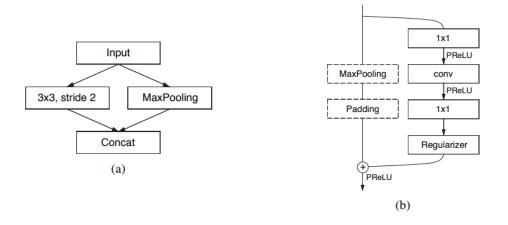
Figure 25: (a) ENet initial block; (b) ENet down-sampling bottleneck block [63]
