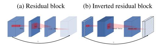
Figure 29: The architecture of (a) a residual block and (b) an inverted residual block [68]
