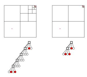
Figure 16: Spatial representation (top) and conceptual representation (bottom) of quadtrees [84]
