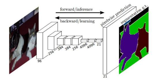
Figure 3: FCN performing semantic segmentation. The number of channels (feature space size) produced by each convolutional layer is indicated [42]
