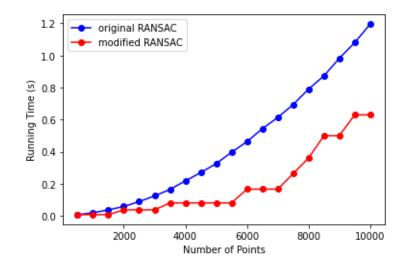
Figure 23: The relationship between the number of points and the running time when  $\sigma = 40$
