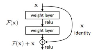
Figure 4: Residual block in ResNet [28]
