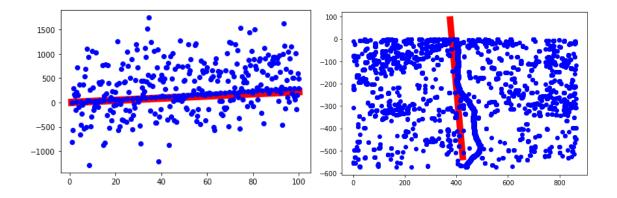
Figure 24: Performance of the modified RANSAC algorithm on detection of a line with Gaussian noise (left) and on detection of points associated to a crack (right)
