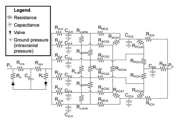
Figure 6. Electrical analog diagram of the cerebral circulation module. All resistances and capacitances are labeled, values and descriptions for which are given in Appendix A1. P<sub>A</sub> is the inlet, given as the arterial pressure value from the systemic model. P<sub>V</sub> is the outlet, given as superior vena cava pressure from the systemic model.
