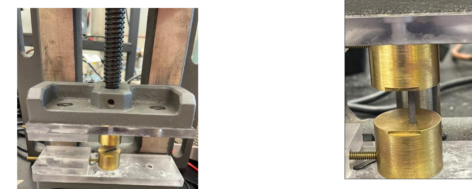
Figure 5: Measurement methods for Transverse Direction (TD) and Flow Direction (FD)
