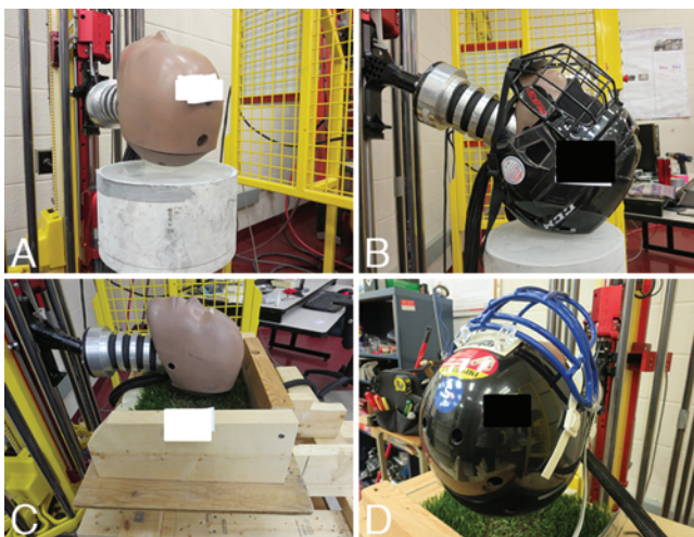
FIG. 1. Monorail impact reconstructions for fall to ice (A), fall to ice in youth ice hockey (B), fall to turf in youth soccer (C), and fall to turf in youth Canadian football (D). Figure is available in color online only.
