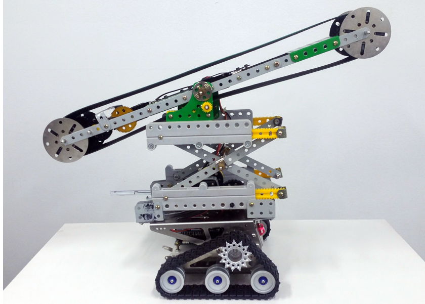
Figure 12: A mobile conveyor belt.
