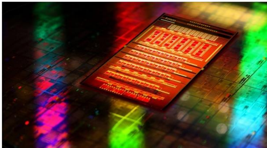
Figure 1.2: IBM's first on-package silicon photonic chips [13].
