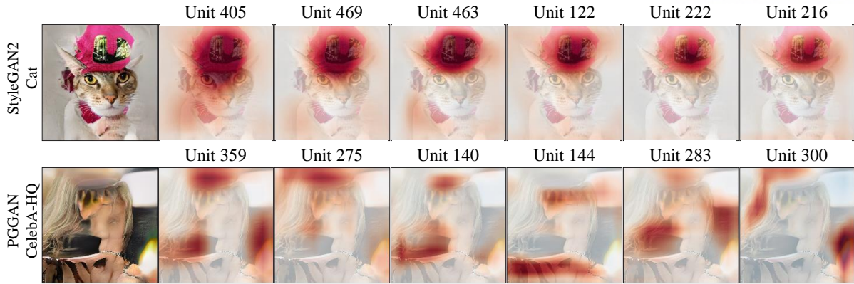
Figure 4.4: An illustrative examples for CLA based artifact generating internal unit identification. Bilinear upsampling for internal units are performed to overlay with the original generation. The red color denotes the high activation values.
