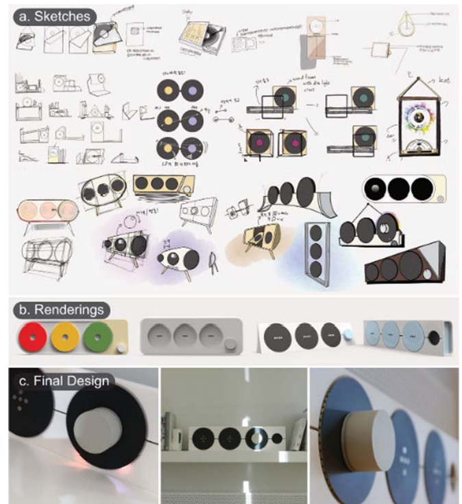
FIGURE 2. Design process of Musée. (a) Variations of concept sketches, (b) renderings or preselected design and (c) Final design.
