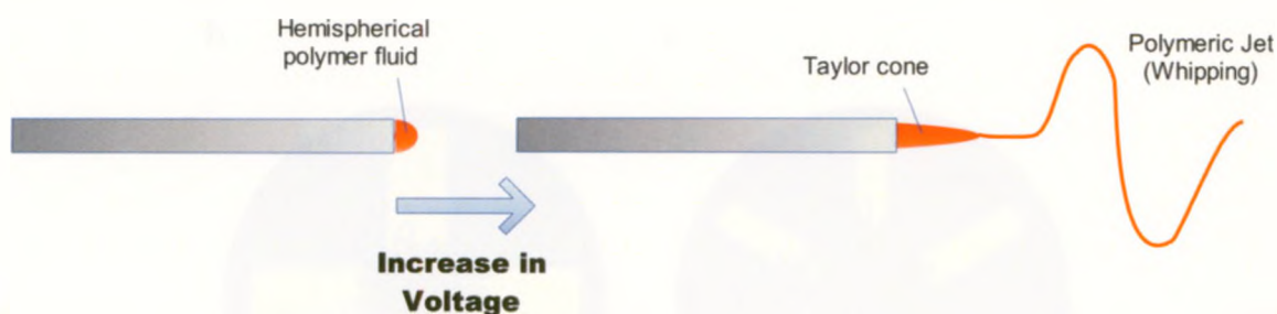
Figure 2.1. (a) Schematic drawing of an electrospinning setup, (b) the process of electrospinning at the tip of a needle.
