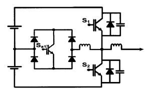
Figure 1.15. The ARCP inverter using one auxiliary switch per phase leg [64]
