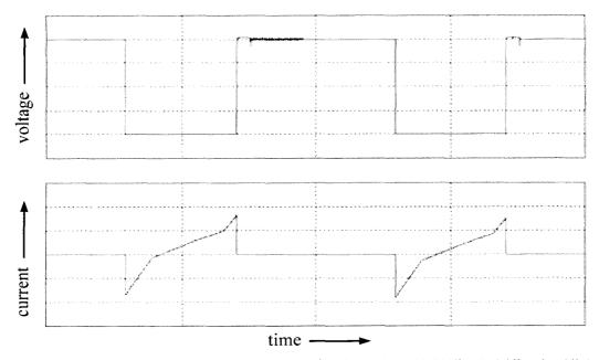
Figure 4.3. Voltage and current wave forms of switch,  $Q_3$  (100 V/div, 3 A/div, 4µs/div)
