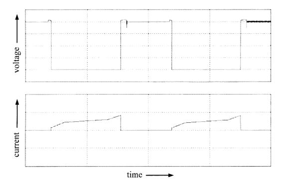
Figure 4.14. Voltage and current wave forms of switch, *Q*<sub>6</sub> (100 V/div, 3 A/div, 4µs/div)
