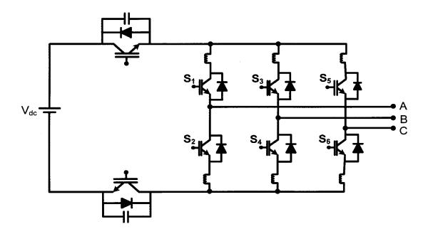
Figure 1.11. DC-rail zero-current switching inverter [46]
