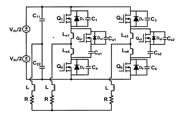
Figure 2.1. Proposed three-phase inverter
