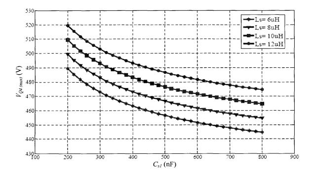
Figure 3.2 Switching stress of switch,  $Q_4$  versus clamping capacitor,  $C_{s1}$
