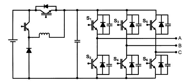
Figure 1.10. DC-rail ZVT inverter [43]
