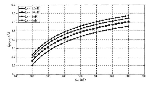
Figure 3.4 Peak current of switch,  $Q_4$  versus clamping capacitor,  $C_{s1}$
