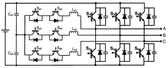
Figure 1.13. The ARCP inverter [54], [55]
