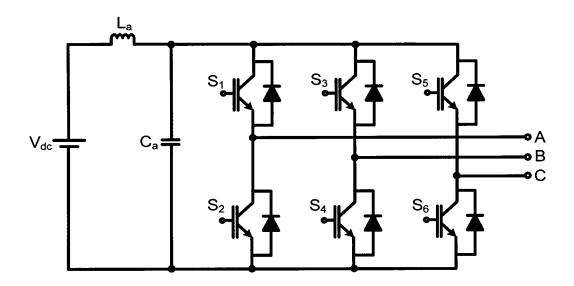
Figure 1.6. The six-switch resonant DC-link inverter [22]
