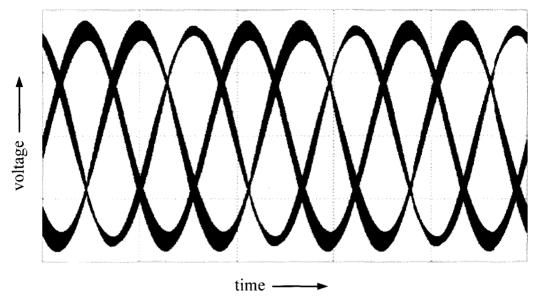
Figure 4.15. Three-phase output voltage (100 V/div, 10 ms/div)
