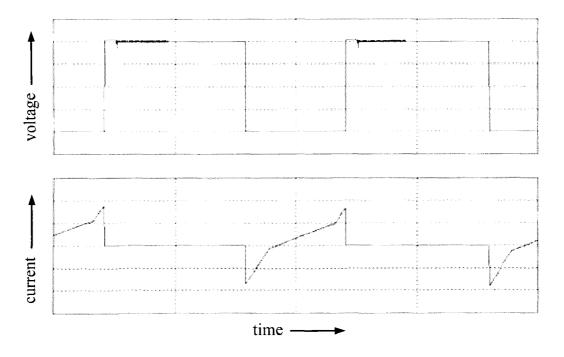
Figure 4.2. Voltage and current wave forms of switch,  $Q_4$  (100 V/div, 3 A/div, 4µs/div)
