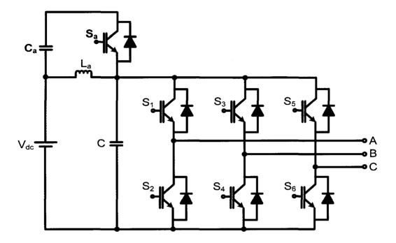
Figure 1.7. Actively clamped resonant DC-link inverter [23]
