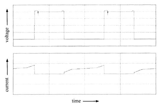
Figure 4.12. Voltage and current wave forms of switch,  $Q_4$  (100 V/div, 3 A/div, 4µs/div)
