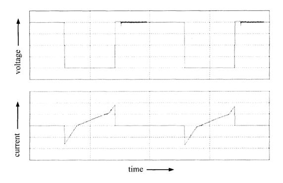
Figure 4.1. Voltage and current wave forms of switch, Q<sub>1</sub> (100 V/div, 3 A/div, 4µs/div)
