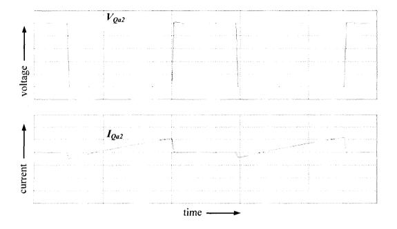
Figure 4.6. Voltage and current wave forms of switch, Qa2 (20 V/div, 4 A/div, 8µs/div)
