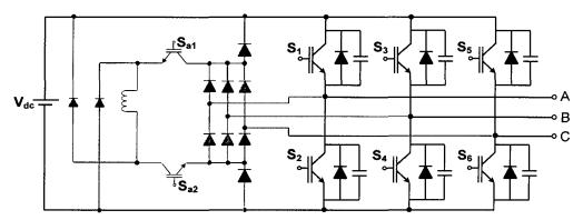
Figure 1.17. The ZVT inverter using two auxiliary switches [68]
