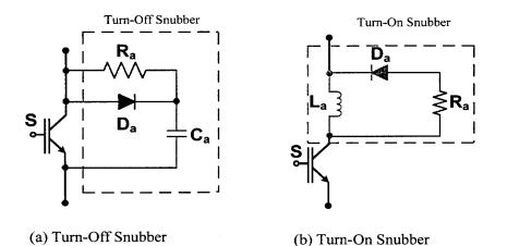
Figure 1.3. Passive RCD and RDL snubbers
