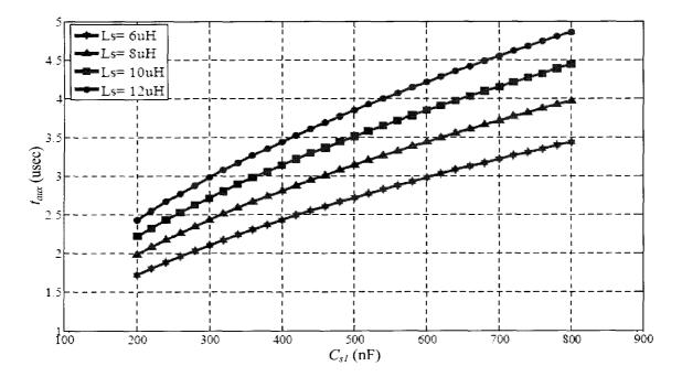
Figure 3.3 On-time of auxiliary switch,  $Q_{al}$  versus clamping capacitor,  $C_{sl}$ 64
