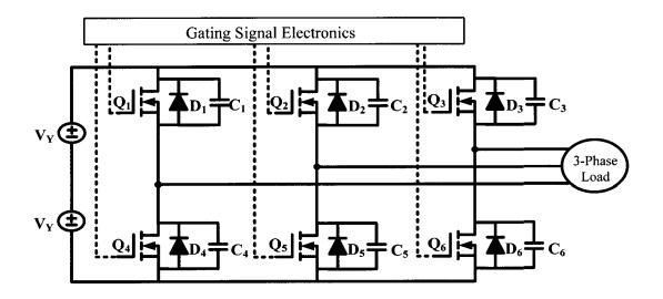
Figure 2.2. Conventional six-switch three-phase inverter
