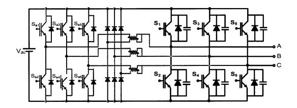
Figure 1.14. The ZVT inverter with coupled inductor feedback [56]
