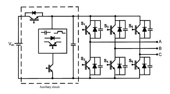
Figure 1.9. Typical configuration of quasi-resonant DC-link inverter
