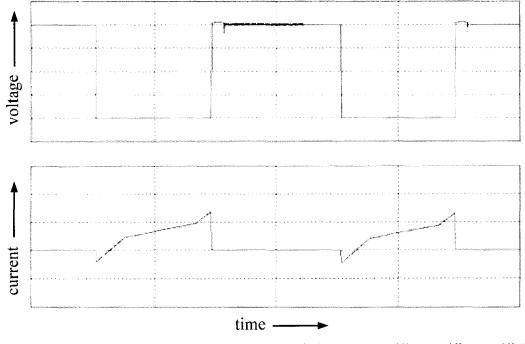
Figure 4.9. Voltage and current wave forms of switch,  $Q_3$  (100 V/div, 3 A/div, 4µs/div)
