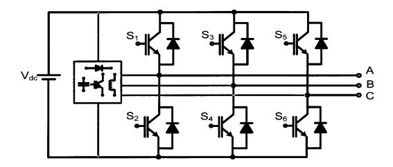
Figure 1.12. Typical configuration of AC-side soft-switching inverter
