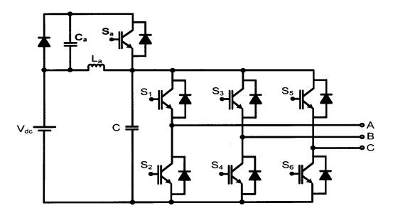
Figure 1.8. Synchronized resonant DC-link inverter [36]
