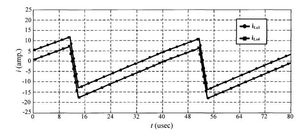
Figure 4.17. Current through  $L_{s1}$  and  $L_{s4}$  (in MATLAB)
