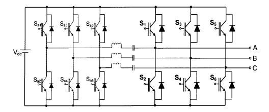
Figure 1.18. The six-switch ZCT inverter
