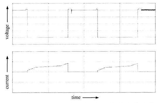
Figure 4.13. Voltage and current wave forms of switch, Q3 (100 V/div, 3 A/div, 4µs/div)
