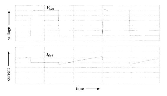
Figure 4.5. Voltage and current wave forms of switch,  $Q_{al}$  (20 V/div, 4 A/div, 8µs/div)
