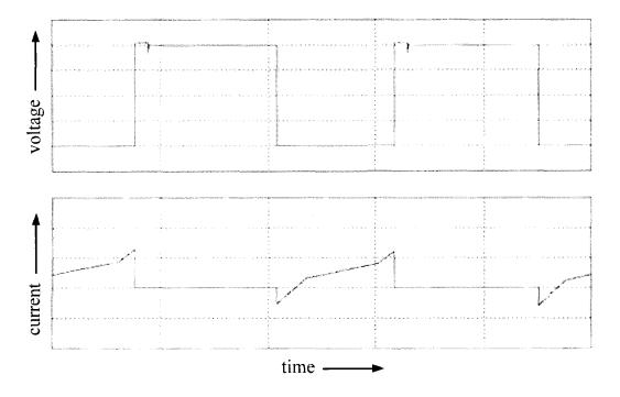
Figure 4.8. Voltage and current wave forms of switch,  $Q_4$  (100 V/div, 3 A/div, 4µs/div)
