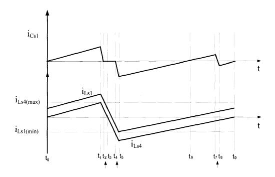
Figure 2.7. Current waveforms of the snubber elements  $C_{sl}$ ,  $L_{sl}$  and  $L_{s4}$
