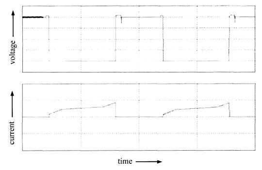
Figure 4.11. Voltage and current wave forms of switch,  $Q_1$  (100 V/div, 3 A/div, 4µs/div)
