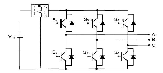
Figure 1.5. Typical configuration of DC-side soft-switching inverter
