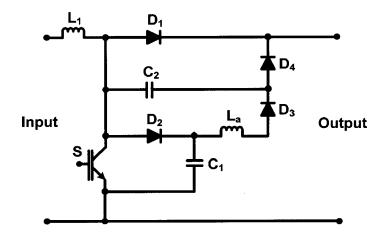
Figure 1.4. Passive lossless snubber
