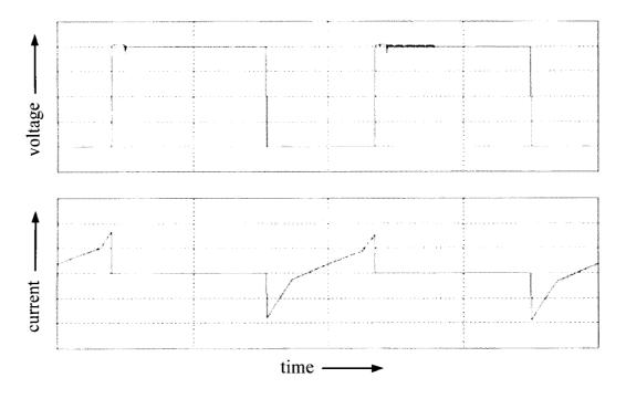
Figure 4.4. Voltage and current wave forms of switch,  $Q_6$  (100 V/div, 3 A/div, 4µs/div)
