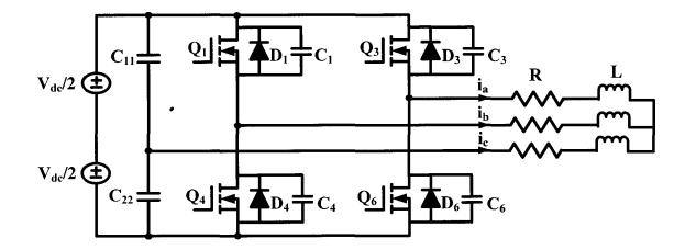
Figure 2.5. Reduced switch three-phase inverter
