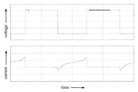
Figure 4.10. Voltage and current wave forms of switch,  $Q_6$  (100 V/div, 3 A/div, 4µs/div)
