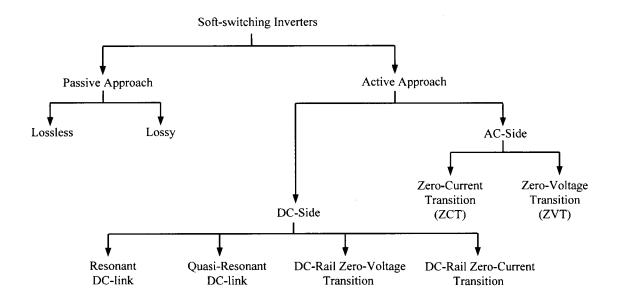
Figure 1.2. Classification of soft-switching inverter techniques
