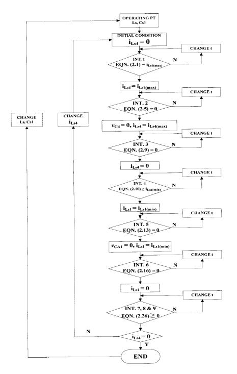
Figure A.1. Flowchart of program to generate real-time graphs of the currents in inductors
