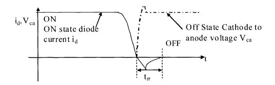
Figure 3.1 Reverse recovery current in a diode.
