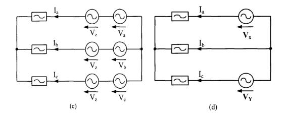
Figure 2.6. Supplying three-phase load from two voltage sources with 60° phase shift
