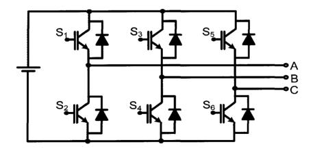
Figure 1.1. The schematic of a three-phase inverter
