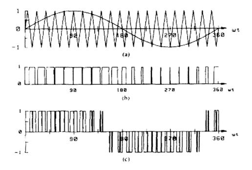
Figure 2.4. Sinusoidal PWM (SPWM). (a)SPWM scheme. (b)VSI switch Q<sub>1</sub> gating signal (c)AC term. [89]
