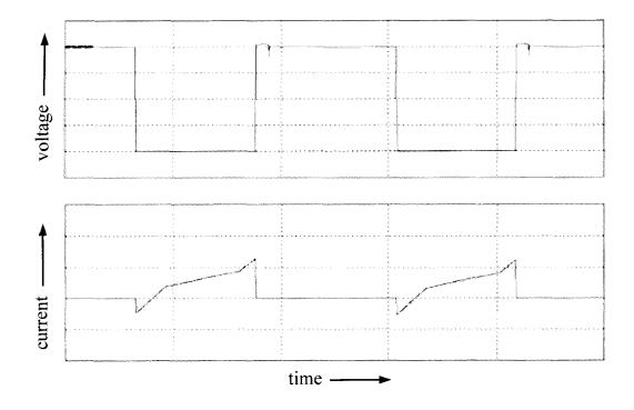
Figure 4.7. Voltage and current wave forms of switch,  $Q_1$  (100 V/div, 3 A/div, 4µs/div)
