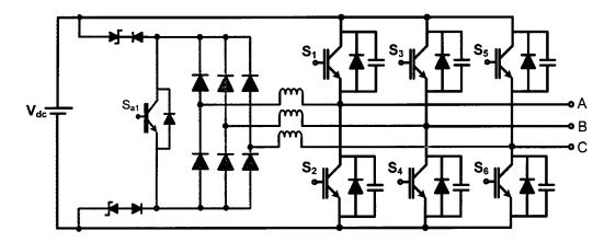
Figure 1.16. The ZVT inverter using one auxiliary switch [67]
