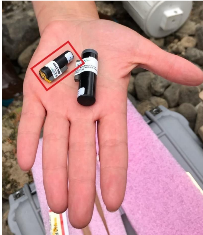
Figure 2 Vemco V9TP-2x-69kHz coded transmitter (indicated by the red box).
