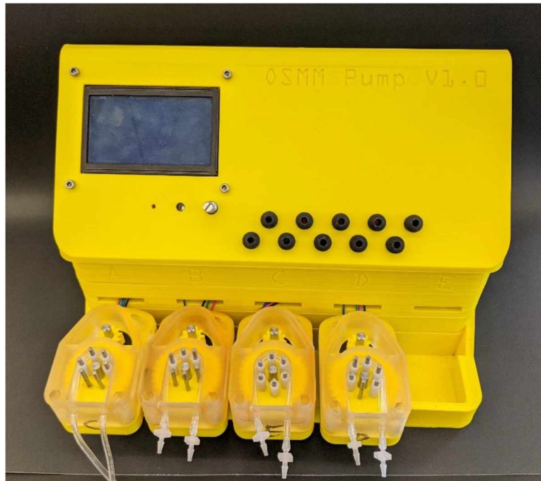
Figure 8: OSMO Pump Control Box
