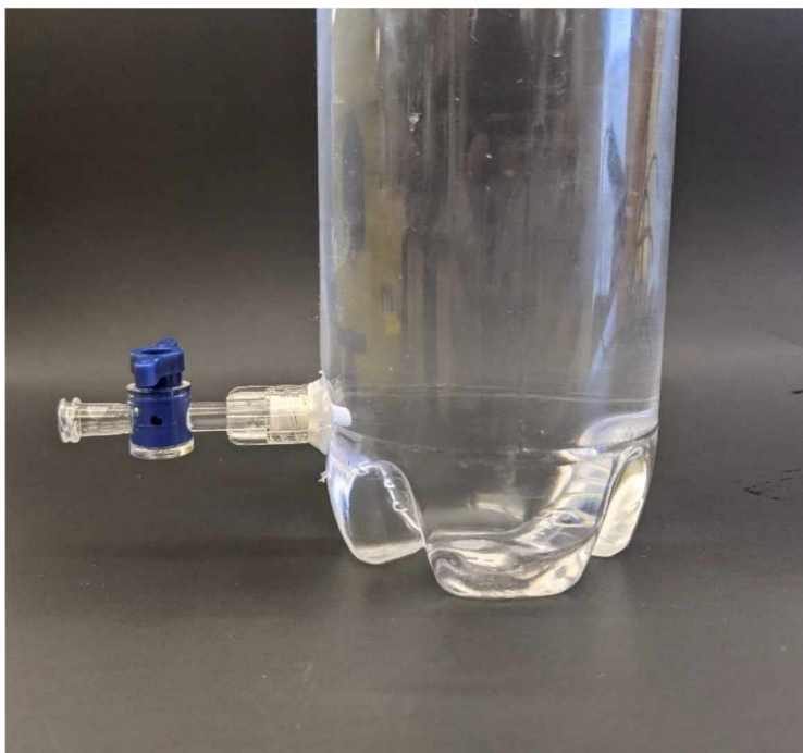
Figure 21: Side view of collection bottle, Luer-lock fitting, and stopcock.
