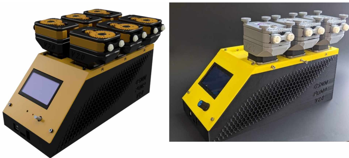
Figure 10: CAD Render of Version 2 Control Box and Pumps (a) and Actual Printed Control Box and 3 Pumps (b)
