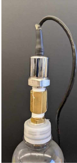
Figure 23: Pressure transducer assembly showing transducer (top), adapter fittings (middle), and collection bottle (bottom).
