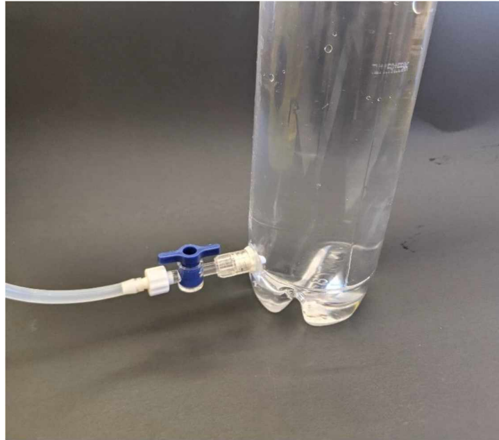
Figure 22: Alternate view of collection bottle, connect to pump tubing
