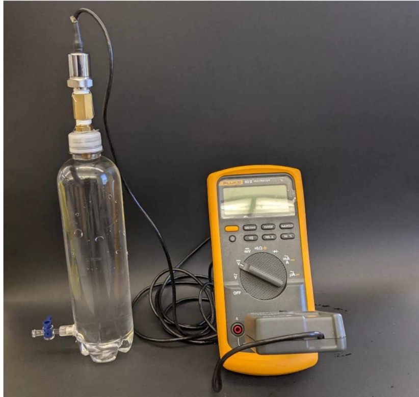
Figure 20: Fluke Multimeter (yellow) and pressure transducer unit (black)
