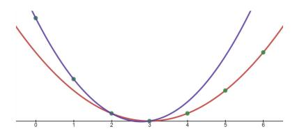
**Figure 1.3** Even with two errors introduced, only the original polynomial can pass through at least five points
