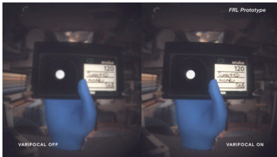
Figure 12: Near viewing in VR with Varifocal turned off and on. 74
