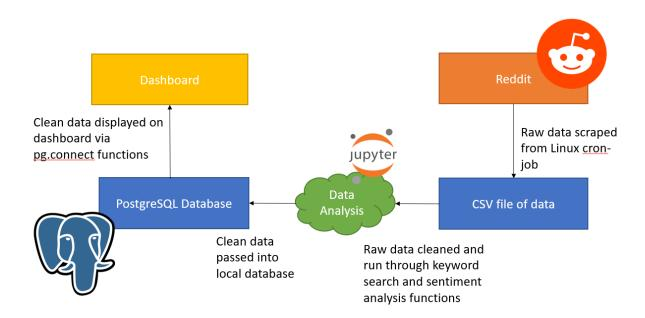
**Figure 6**: Flow chart depicting process for collecting data, cleaning/analyzing data, and finally displaying the data.
