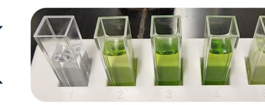
Read absorbance at 470nm, 649nm, 664nm & 750nm by UV-Vis spectroscopy
