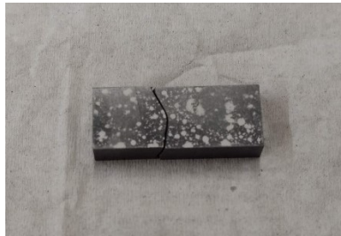
Figure B.14 Typical specimen failure after test run
