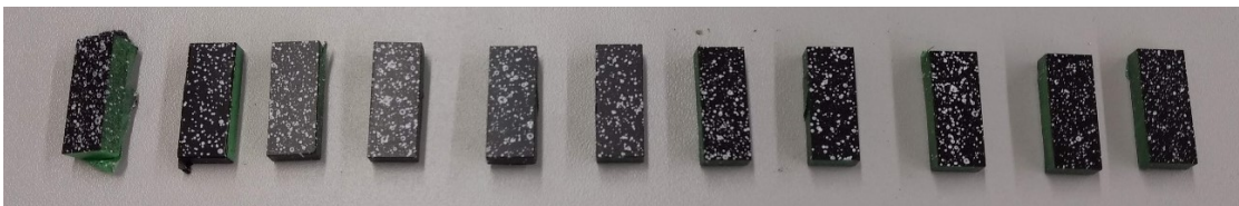
Figure 6.7 Si 3 N 4 specimens prepared with white-on-black speckle pattern for DIC
