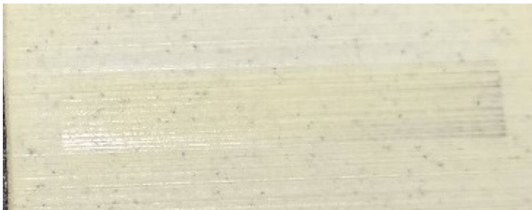
Figure 6.17 TBC friction marks after test run.
