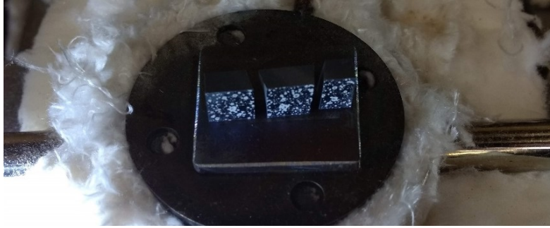
Figure 6.14 Failed specimen segments in test rig after test run; broken segments are purposely spaced further apart to show failure
