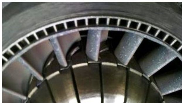
Figure 3.11 Silicon nitride blades speckled with melted combustor debris (DOD) after preliminary testing at a TIT of 720 °C and tip speed of 300 m/s
