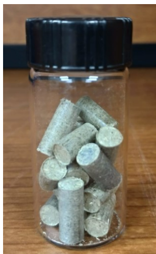
Figure A.2 Hemp pellets produced through the single pellet system
