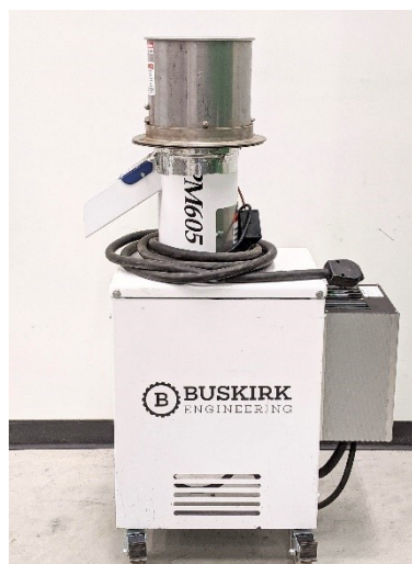
Figure 3.4 The PM605 (Buskirk Engineering) laboratory-scale pellet mill used for the production of lignin pellets
