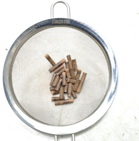
Figure 4.4 Poplar wood lignin pellets produced with lignin originally having a 6.14% moisture content using a single pellet system.
