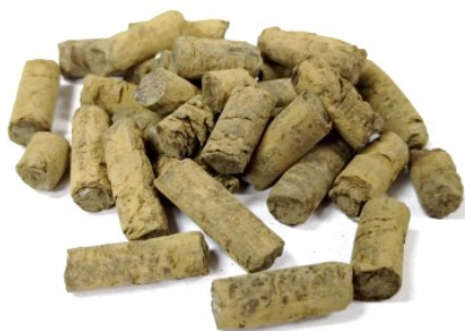
Figure 4.5 Corn stover lignin pellets produced with lignin originally having a 10.64% moisture content using a single pellet system.
