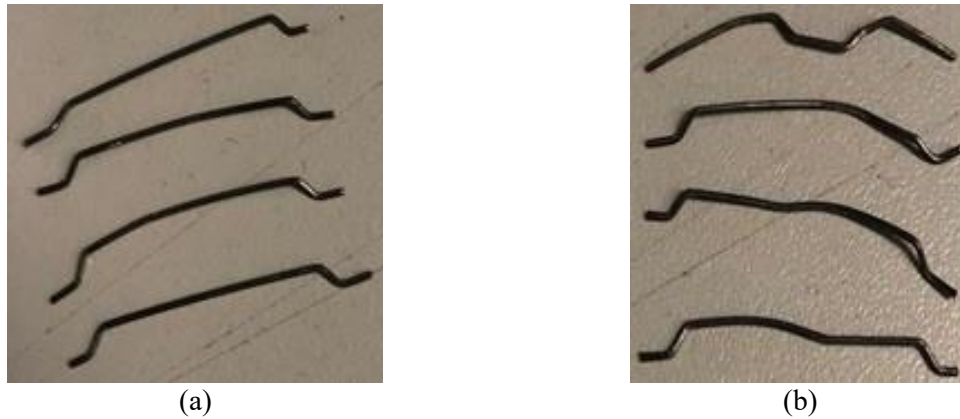
Figure 5-16 Deformed fibers after DPD measurements of F-A mixtures proportioned with (a) MSA20-1 and (b) MSA20-2 coarse aggregate mixtures.
