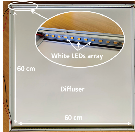
Figure 3.6 Typical LED light fixture used for indoor illumination (Sylvania START Panel Flat UGR19 600x600 Neutral White) consisting of 144 total mid-power LEDs and providing a luminous flux of 3500 lm.
