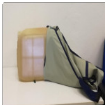
Fig 2: Mesurement of the absorbed dose with lead protection around the phantom.
