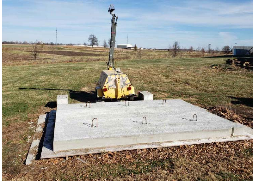
Figure 4-8: The concrete specimen laying on the ground with the IR-UTD system located at the north side.
