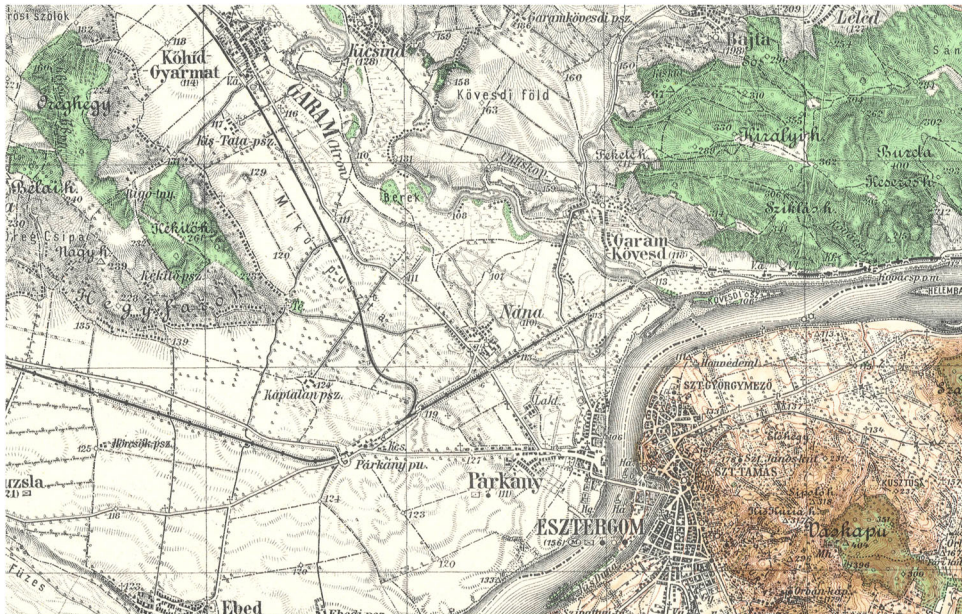
Figure 3. The 4861 sheet (1:75,000 scale) published in 1933. We can recognise that the relief representation on the Czechoslovakian part (the larger, NW part of the inset) is still shown with Lehmann hachures, while on the Hungarian section (SE part of the inset) the relief is represented by contour lines. The whole content on the Czechoslovakian side (including the lettering) based on the Third Military Survey.
