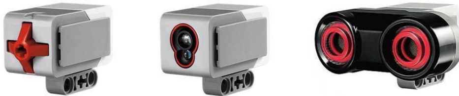
Figure 5: EV3 Touch sensor, Colour sensor, Ultrasonic sensor 4
