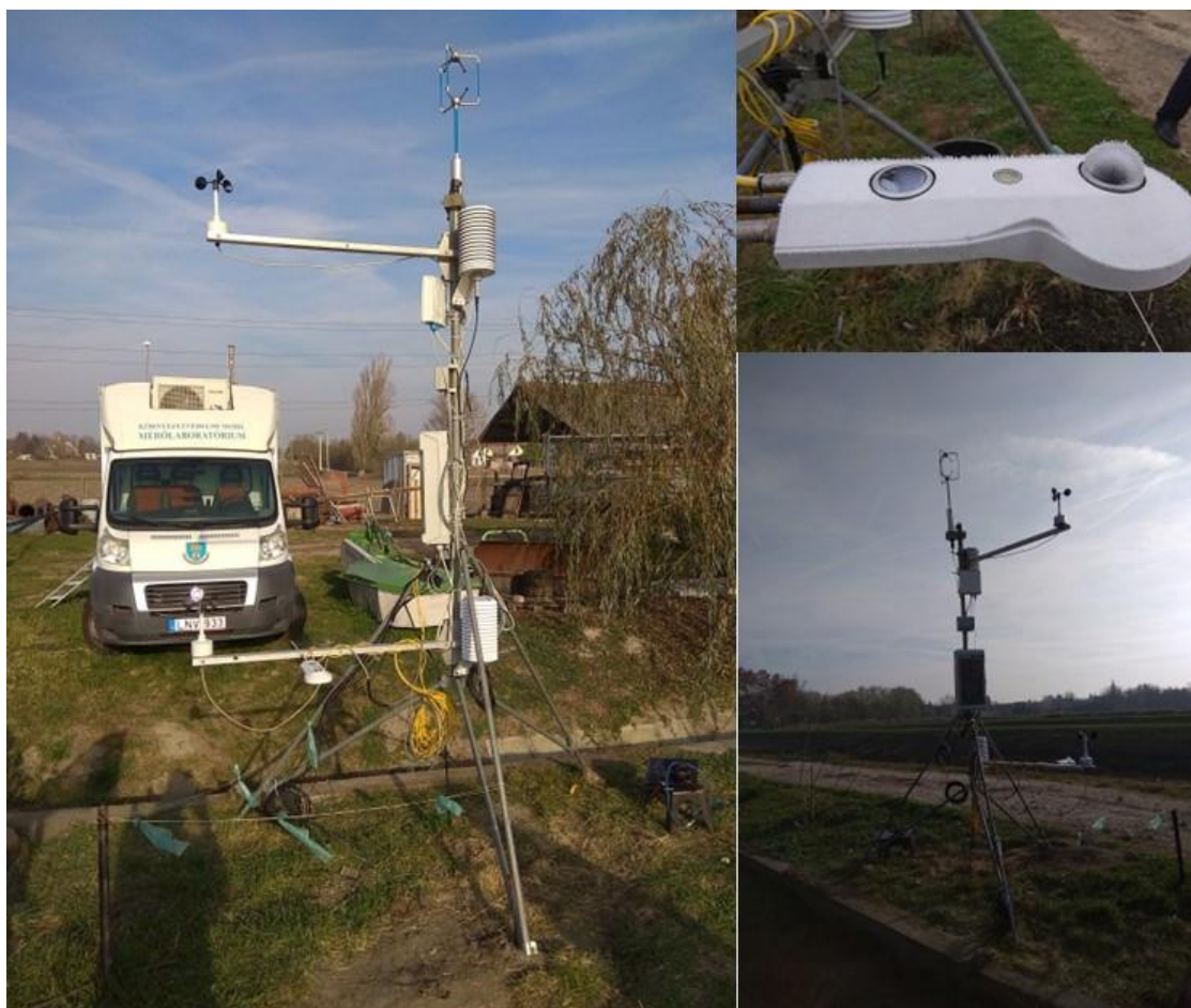
Figure 2. Micrometeorological observation pole and its instrumentation (CNR4 net radiometer, Gill sonic anemometer, temperature, relative humidity, and wind speed gradients). Mobile air chemistry laboratory of the University of Pannonia in the background.
