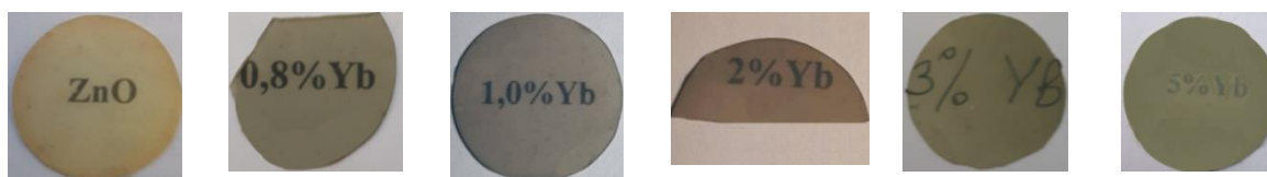
Figure 1. Photographs of undoped and \text{Yb}^{3+} -doped ZnO transparent ceramics with increasing Yb doping level (from left to right). The labels indicate the Yb concentration (in wt%).
