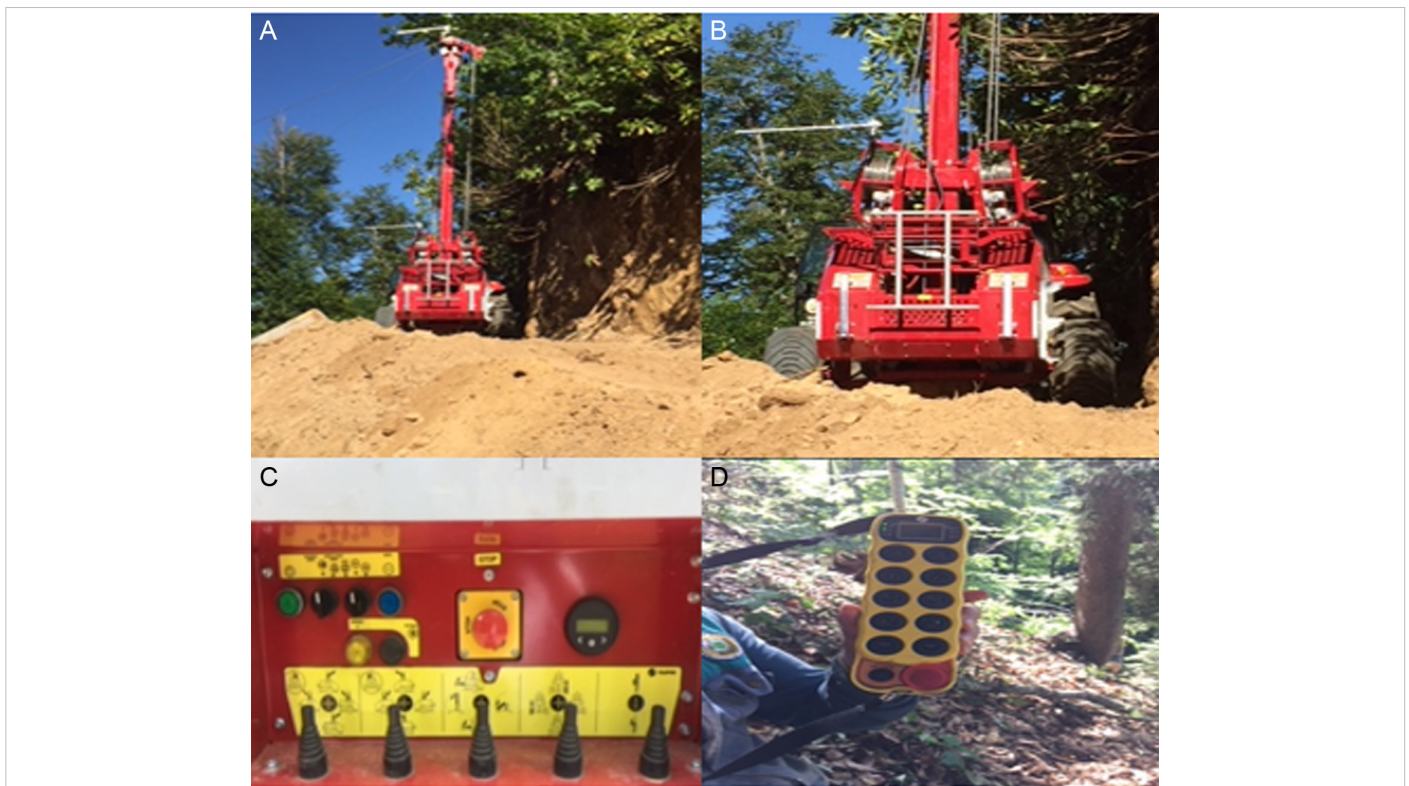
Figure 2. (A and B) Tajfun MOZ 500 GR Cable Yarder ; (C) outer Panel ; (D) Control Panel .
