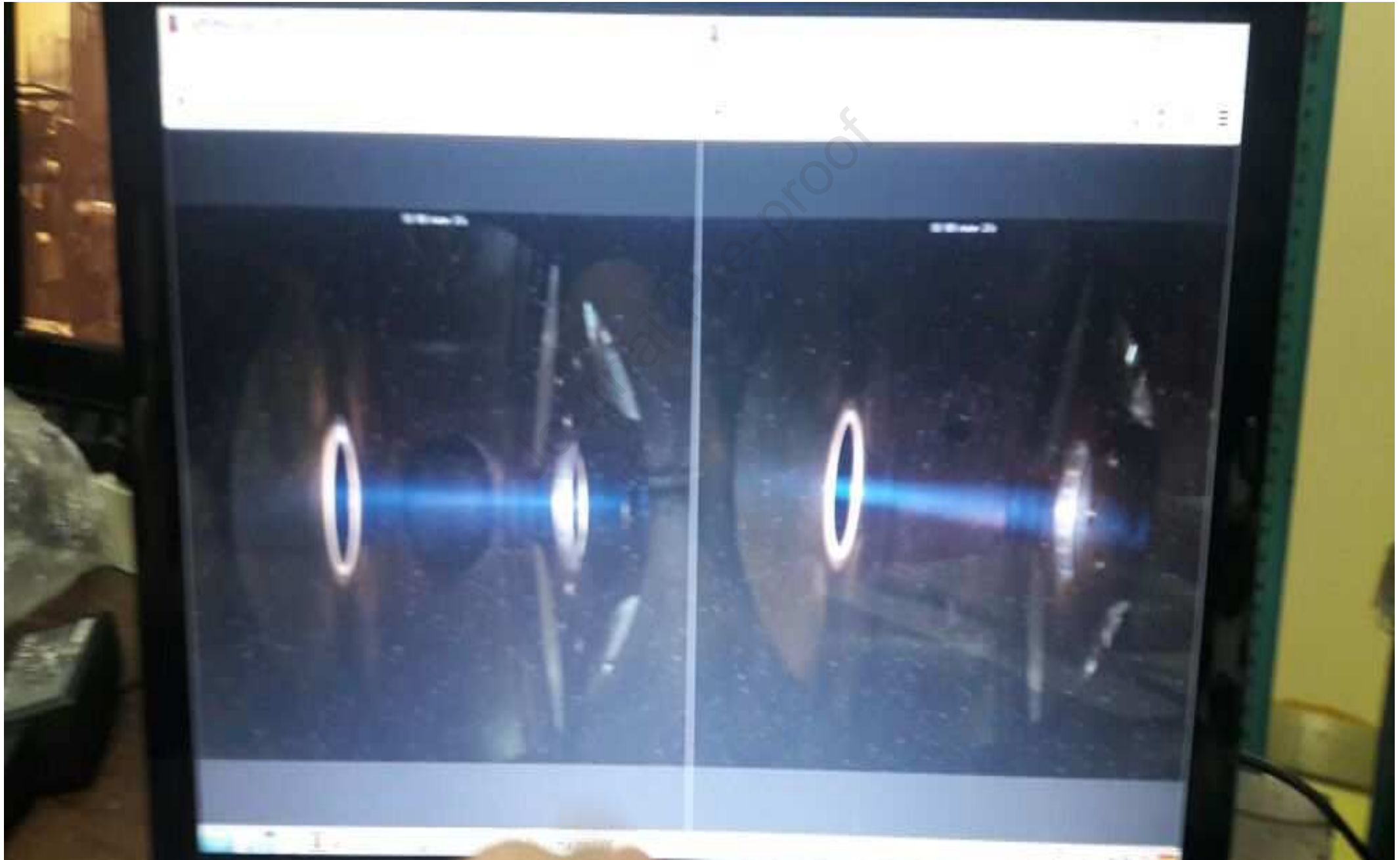
Journal Pre-proof Fig. 2 Proton beam of 0 nA entering into the Faraday cup (two views in the perpendicular xz & yz planes, z being the beam propagation direction).
