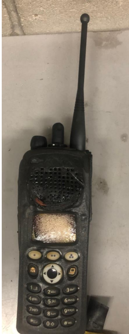
Figure 0.19: Radio C Damage After Pocket Test R3
