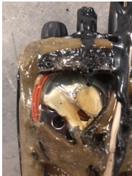
Figure 0.33: Radio A.1 Damage Close Up After Pocket Test #6
