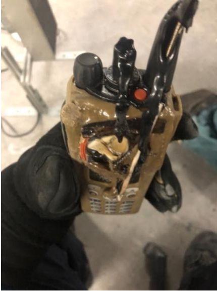
Figure 0.34: Radio A.1 Top Damage After Pocket Test #6
