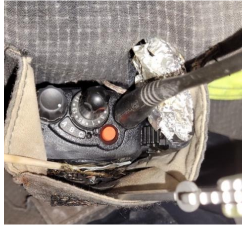
Figure 0.25: Radio C.1 Top View after Pocket Test #5 Prior to Removal
