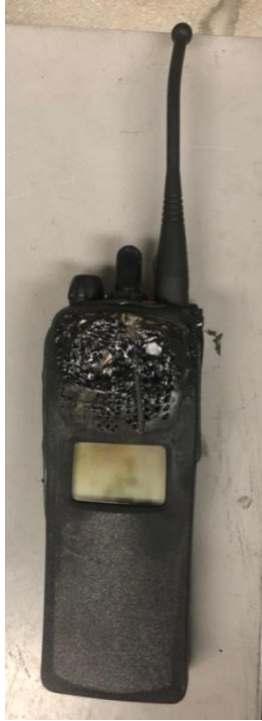
Figure 0.62: Radio E.6 Damage After Removal After 12 Strap Outside Test #1
