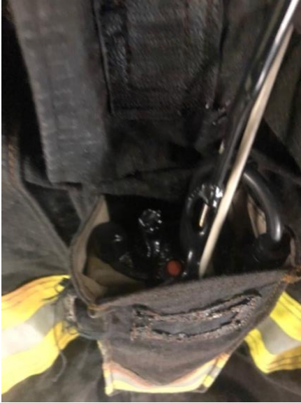
Figure 0.30: Radio A.1 Damage Prior to Removal After Pocket Test #6
