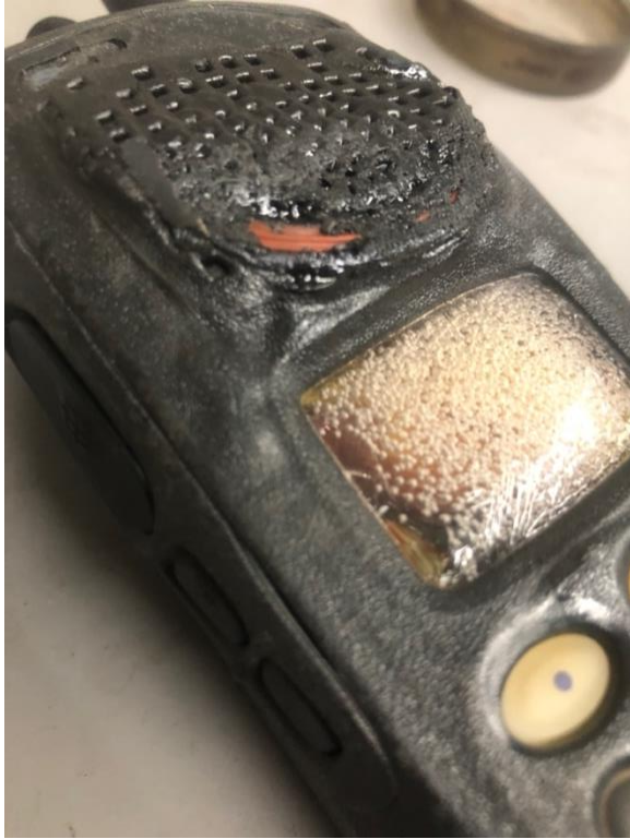
Figure 0.20: Radio C Melting After Pocket Test R3
