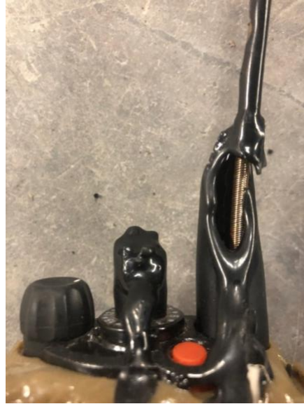
Figure 0.35: Radio A.1 Knob and Antenna Melting After Pocket Test #6
