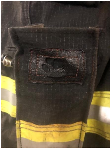
Figure 0.68: Turnout Coat Radio Pocket Closure Degradation after Pocket Test #1
