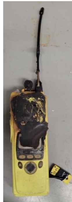
Figure 0.16: Radio B Damage After Removal
