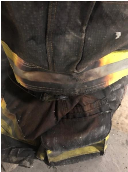
Figure 0.73: Trim Degradation and Turnout Gear Discoloration
