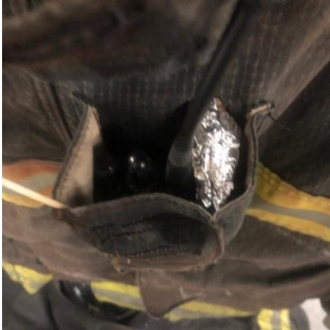
Figure 0.24: Radio C.1 Damage After Pocket Test #5 Prior to Removal
