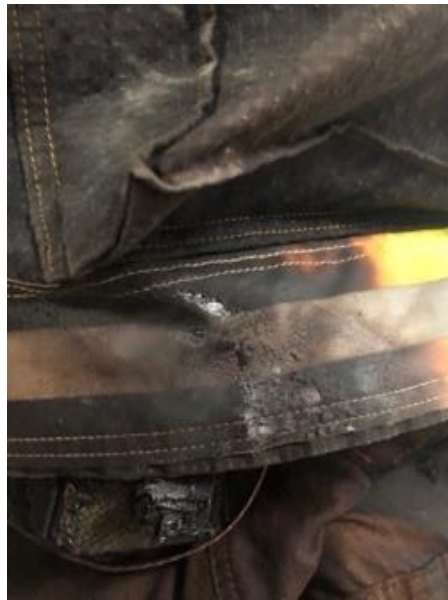
Figure 0.74: Trim Damage After Strap Tests
