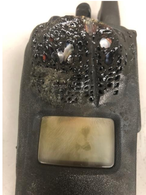
Figure 0.64: Radio E.6 Melting Close Up After 12 Strap Outside Test #1
