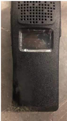
Figure 0.51: Radio E.4 Thermal Damage After 12 Strap Test #2
