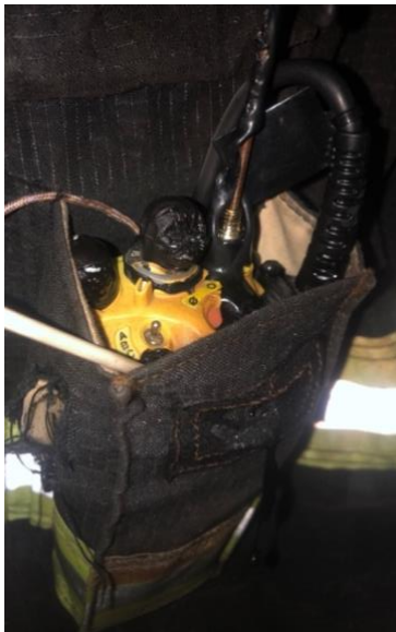
Figure 0.15: Radio B Close Up Damage Prior to Removal
