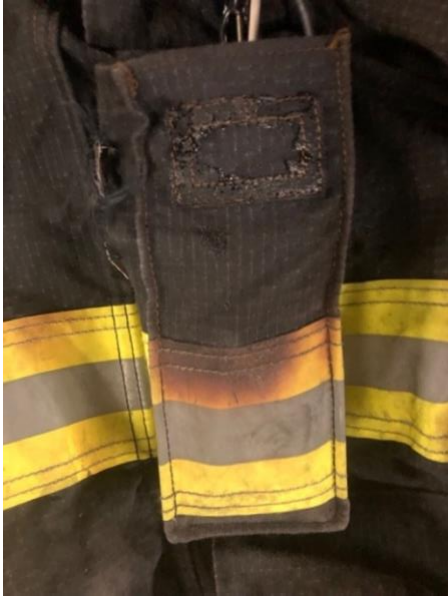
Figure 0.71: Radio Pocket Closure Completely Degraded
