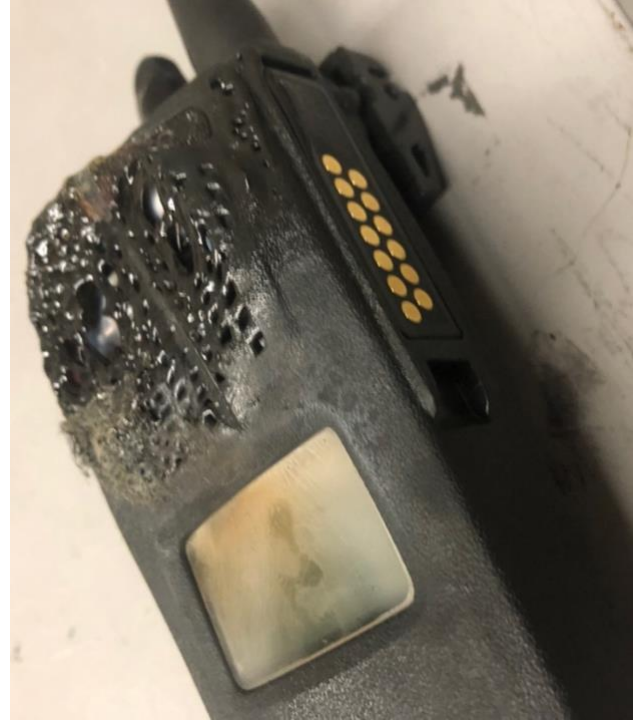
Figure 0.63: Radio E.6 Melting After 12 Strap Outside Test #1
