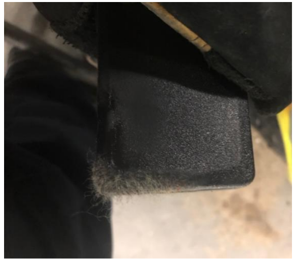
Figure 0.52: Radio E.4 Thermal Damage After 12 Strap Test #2 Close Up
