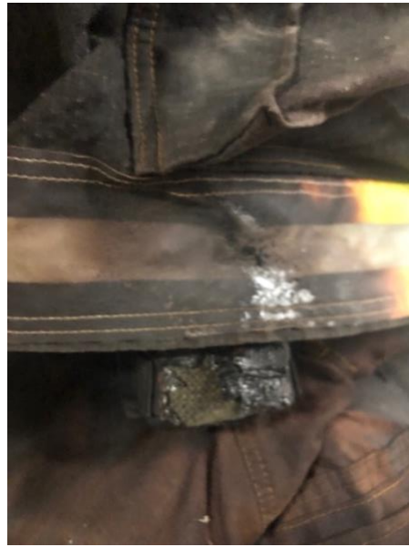
Figure 0.69: Radio Strap and Reflective Trim Damage
