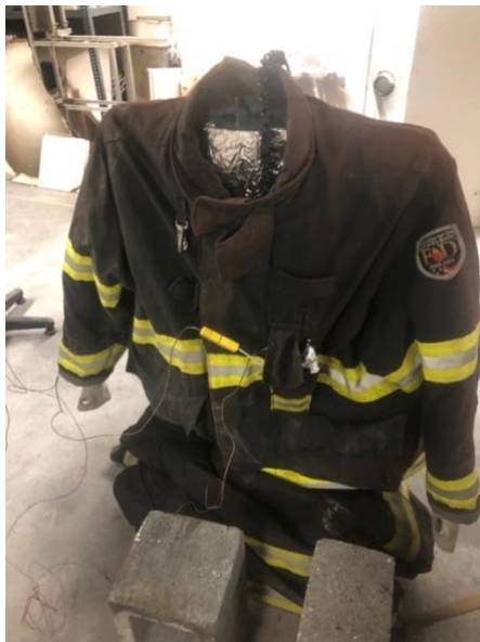
Figure 0.1: Radio Pocket Testing Setup Front View
