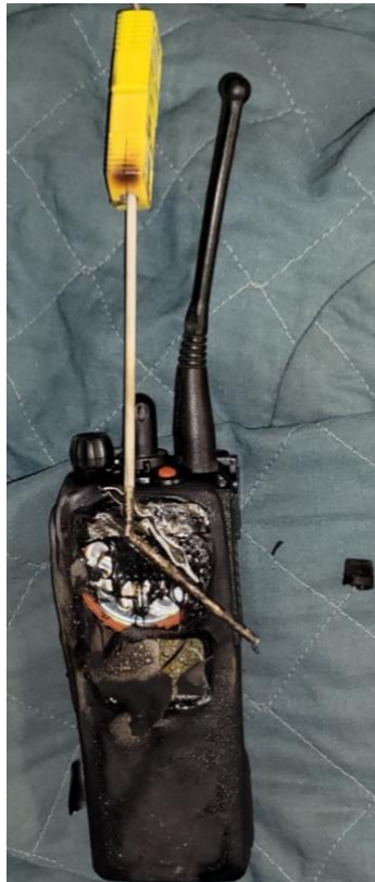
Figure 0.26: Radio C.1 and Thermocouple Damage After Removal After Pocket Test #5
