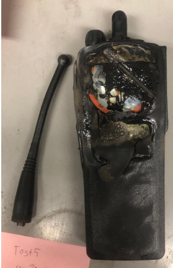
Figure 0.27: Radio C.1 and Antenna Damage After Removal After Pocket Test
