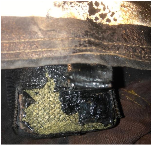
Figure 0.67: Nylon Radio Strap Label Melted After Testing
