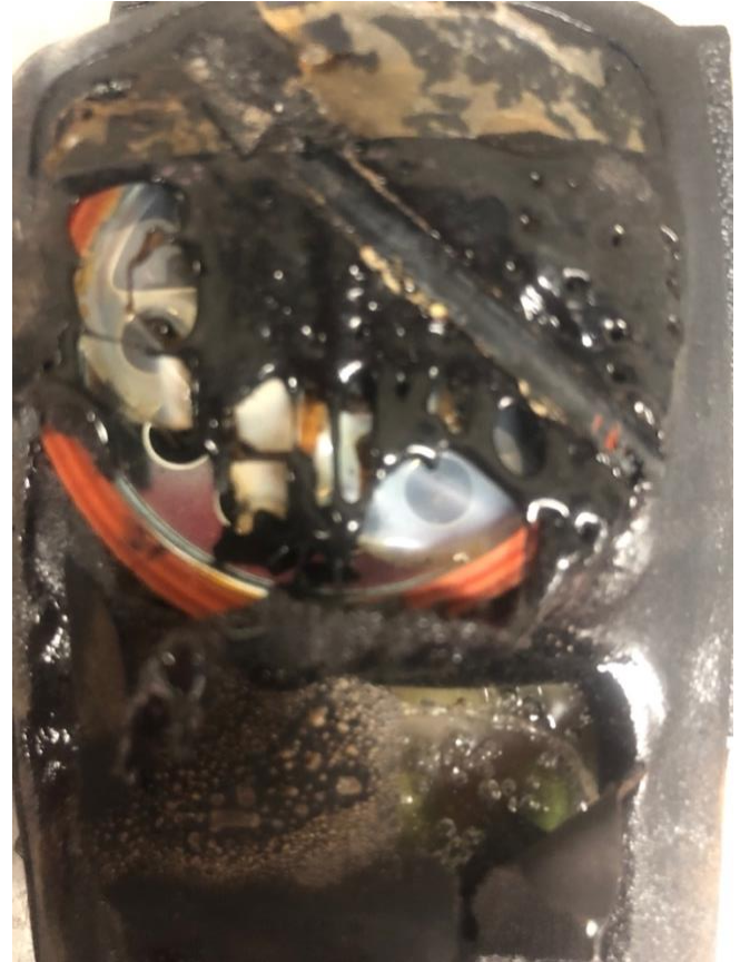
Figure 0.28: Radio C.1 Damage Close Up After Pocket Test #5
