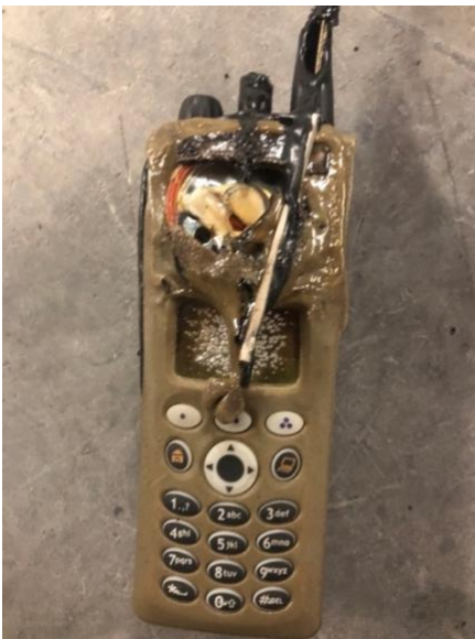
Figure 0.32: Radio A.1 Damage Post Removal After Pocket Test #6
