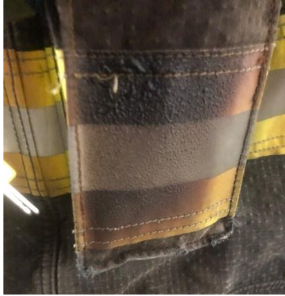
Figure 0.72: Radio Pocket Trim Degradation
