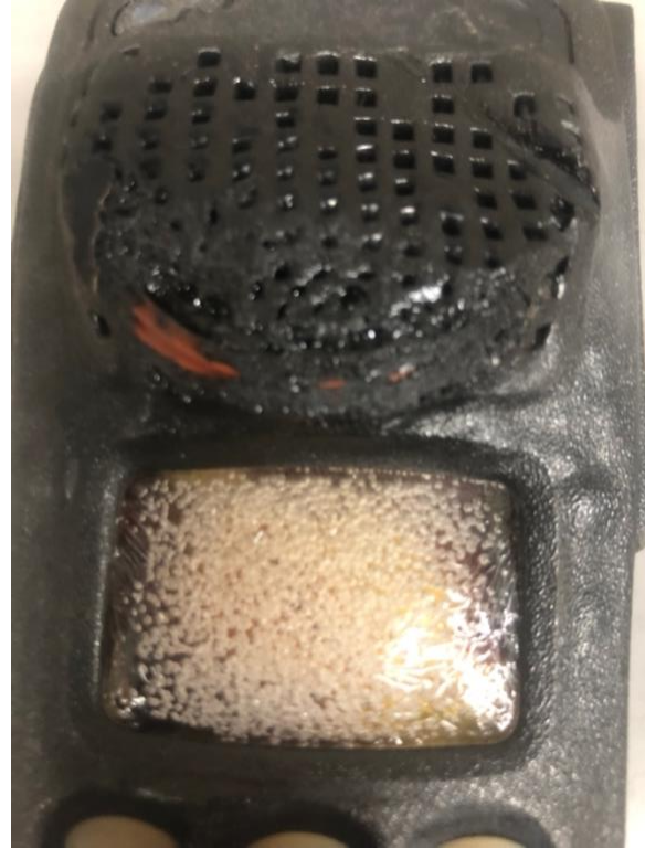
Figure 0.21: Radio C Screen Crazing After Pocket Test R3
