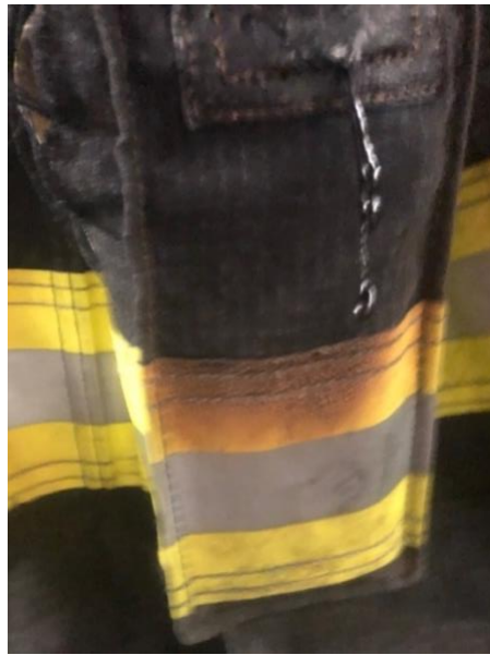
Figure 0.70: Radio Pocket Closure Dripping After Pocket Test #2
