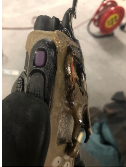
Figure 0.31: Radio A.1 Damage Post Removal After Pocket Test #6
