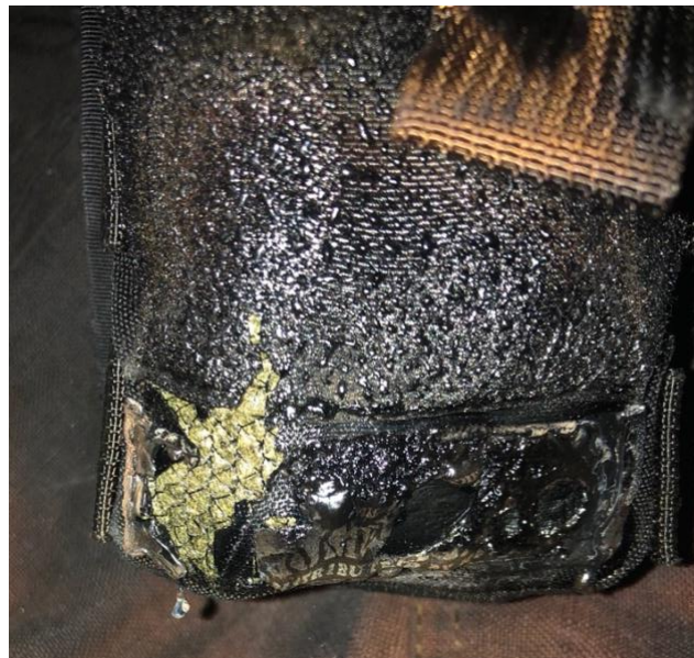
Figure 0.66: Radio Strap Degradation Between Tests
