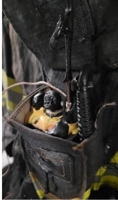
Figure 0.14: Radio B Antenna and Knob Melting
