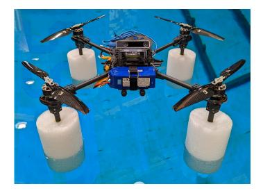
Figure 2.1: Image of the amphibious quadrotor UAV
