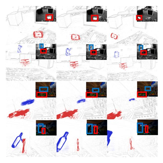
Figure 3.5: Qualitative Evaluation of our method on three datasets. Top two rows: EV-IMO dataset, Bottom two rows: MOD dataset. Insets show the corresponding grayscale/RGB images for reference. The cluster membership is color coded where gray color indicates background cluster. Bounding boxes on the images are color coded with respect to the objects for reference.
