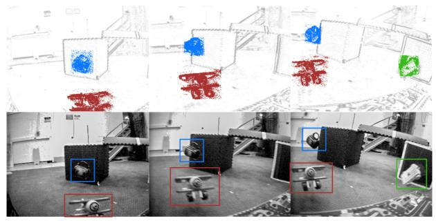
Figure 3.1: Multi-Motion Segmentation with a monocular event camera on an EV-IMO dataset sequence. Top Row: The event frames are color-coded by cluster membership. The corresponding grayscale frames are shown in the bottom row. Bounding boxes on the images are color coded with respect to the objects for reference. *Note that grayscale images are not used for computation and are provided for visualization purposes only*.
