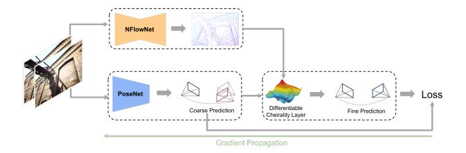
Figure 2.3: Overview of our proposed *DiffPoseNet* framework. Our network starts with a novel normal flow estimation network *NFlowNet* and a first coarse pose estimate. Next, fine pose is estimated using the proposed differentiable cheirality layer.
