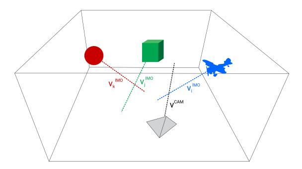
Figure 3.4: Velocity vectors  $v^{\text{CAM}}$  and  $v^{\text{IMO}}_i$  used for data stratification in the MOD++ dataset.
