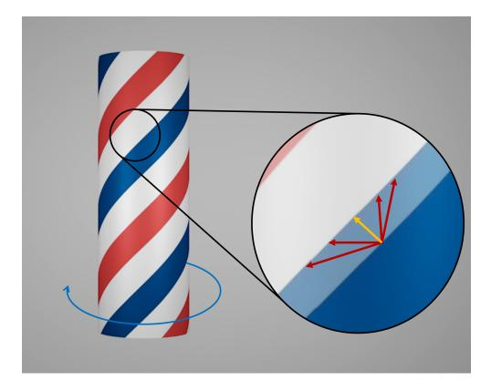
Figure 1.3: The illustration of aperture problem using Barbers' Pole. Line feature observed through a small aperture. It is not possible to determine exactly where each point has moved to. However, normal flow (yellow arrow), the optical flow (red arrow) component perpendicular to the line feature can be computed.
