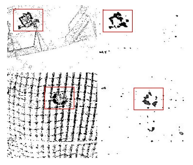
Figure 4.6: Results showing motion segmentation generalization without fine-tuning or re-training on real world data. *SpikeMS* is able to segment the moving object from the scene even in the presence of substantial background noise. The objects in the red bounding box are the true moving objects. Top row: A fast drone approaching a moving event camera. Bottom row: Moving object behind netted background.
