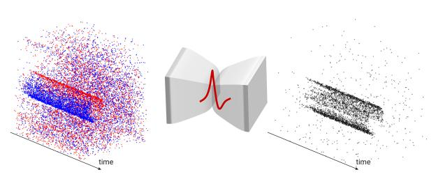
Figure 4.1: Event-based motion segmentation pipeline using a deep spiking neural network. Left to right: Event stream input represented as red (brightness increase) and blue (brightness decrease), representation of the proposed encoder-decoder spiking neural network called *SpikeMS* and the output predicted spike containing only the region of moving object(s).
