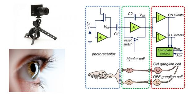
Figure 1.4: Three-layer model of a human retina and corresponding event sensor pixel circuitry [4]
