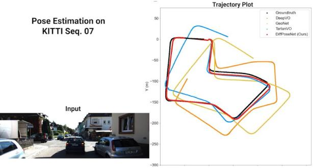
Figure 1.5: *DiffPoseNet*: Egomotion estimation with normal flow and learning from geometry paradigm.
