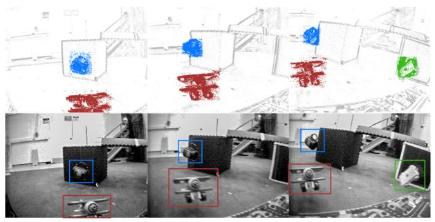
Figure 1.6: *0-MMS*: IMO Segmentation with a monocular event camera on an EV-IMO dataset sequence.
