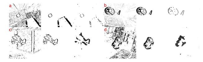
Figure 4.4: Qualitative Evaluation of our approach on two datasets. Top row (a and b): MOD dataset, Bottom row (c and d): EV-IMO dataset. Each sample includes, (left to right) event stream, groundtruth, and network prediction. Here, we show event projections for clarity purposes but *SpikeMS* predicts spatio-temporal spikes.
