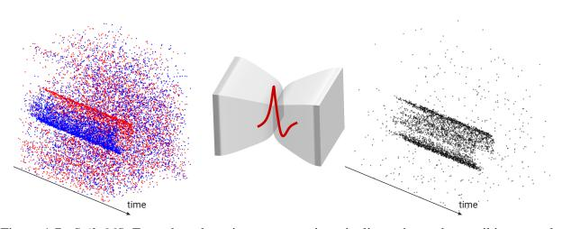
Figure 1.7: *SpikeMS*: Event-based motion segmentation pipeline using a deep spiking neural network.
