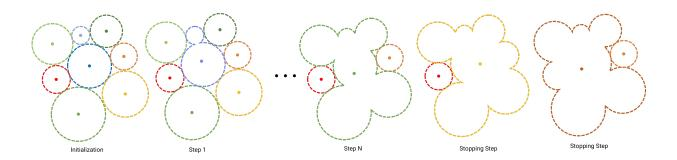
Figure 3.3: Iterative model fitting and merging approach. The colors indicate the average temporal gradient for that particular cluster. (Blue indicates a low value and red indicates a high value). We stop merging whenever the average temporal gradient increases drastically after a merging step since this indicates a merger of the background with an IMO cluster.
