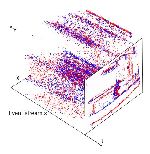
Figure 4.3: Representation of event stream  $\mathcal{E}$  and its corresponding projection (event frame). Note that, only event streams are fed to *SpikeMS*. The event frame is shown only for clarity purposes.
