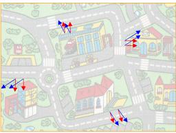
Figure 1.2: The comparison of normal flow vs. optical flow fields. Left: A drone with a down-facing camera is landing vertically on a carpet. Right: Red arrows indicate normal flow, and blue arrows indicate optical flow. The normal flow is the projection of optical flow on the component perpendicular to the edges.
