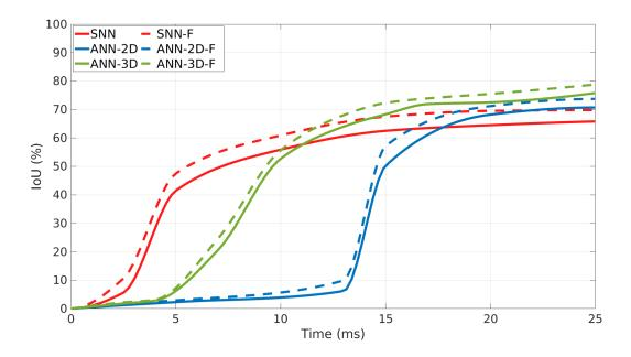
Figure 4.5: Incremental Prediction: Segmentation accuracy vs. input spike window length in milliseconds for various simulation time width  $\Delta t$ . SpikeMS is able to achieve good accuracy significantly faster than ANNs, given smaller input data. The dashed lines represent accuracy improvement after employing a filtering (See Sec. 4.4.3).
