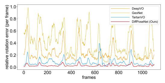
Figure 2.6: Comparison between our model and pure learning based VO on relative rotation error (in °/frame) from KITTI - 07.
