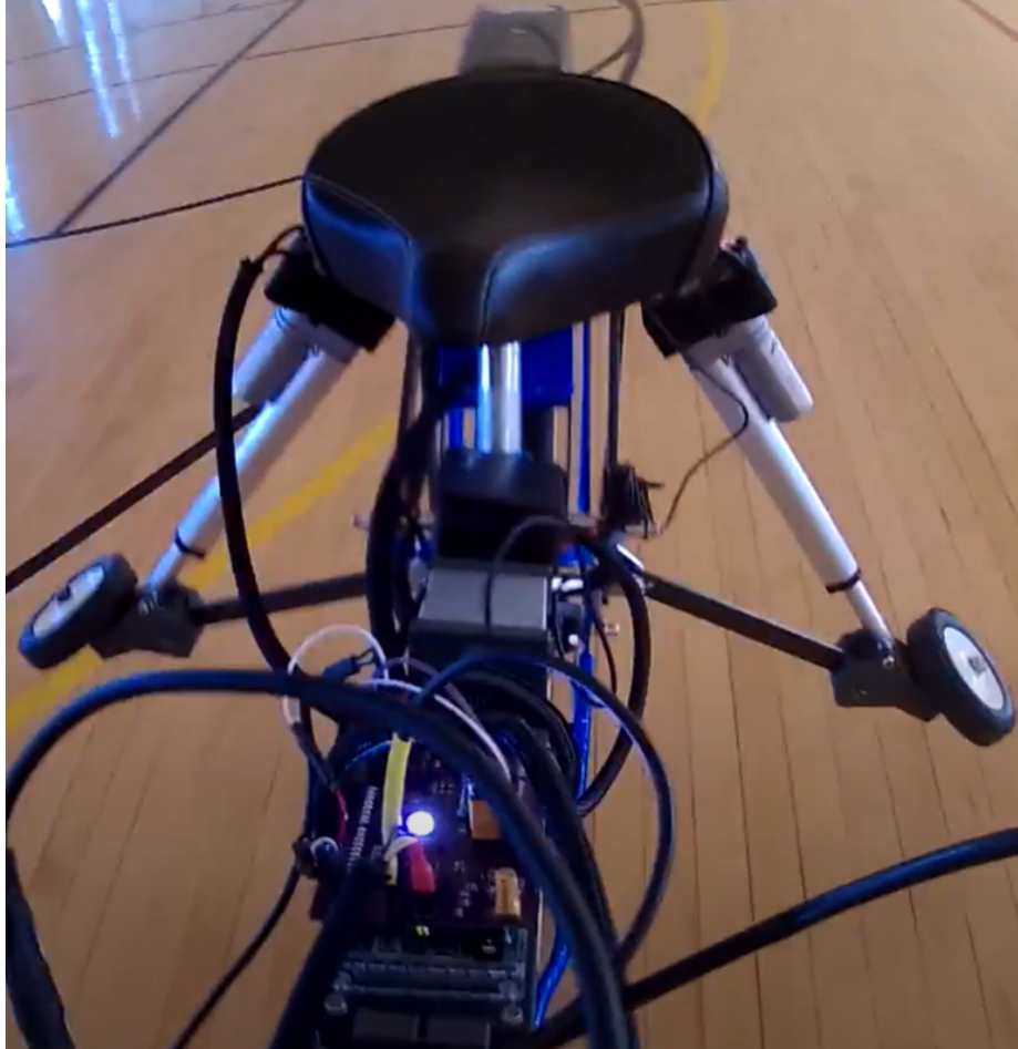
Figure 3.11: When the bike reaches a stable travel speed, actuators retract the ZSS. This figure depicts the ZSS mid-retraction.
