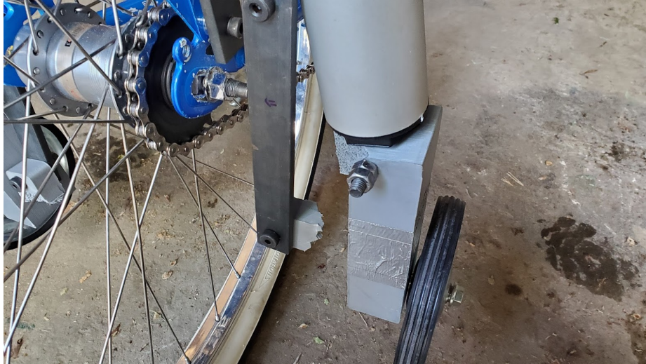
Figure 5.3: PLA proved to be too weak to sustain the loads placed on the block during actuation. Future designs would be fabricated out of nylon.
