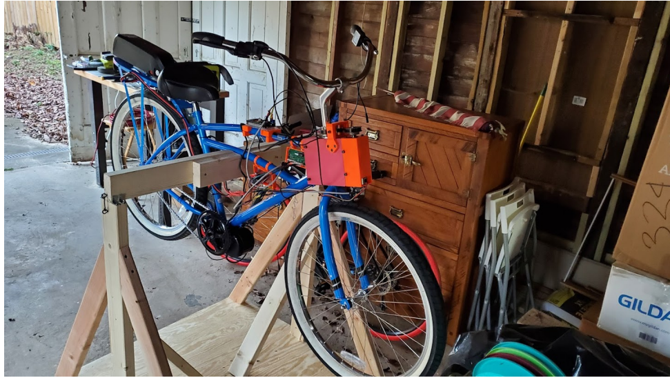
Figure 4.7: Pictured is the configuration of the Autocycle during initial field testing. It is resting on the test stand constructed by the team.
