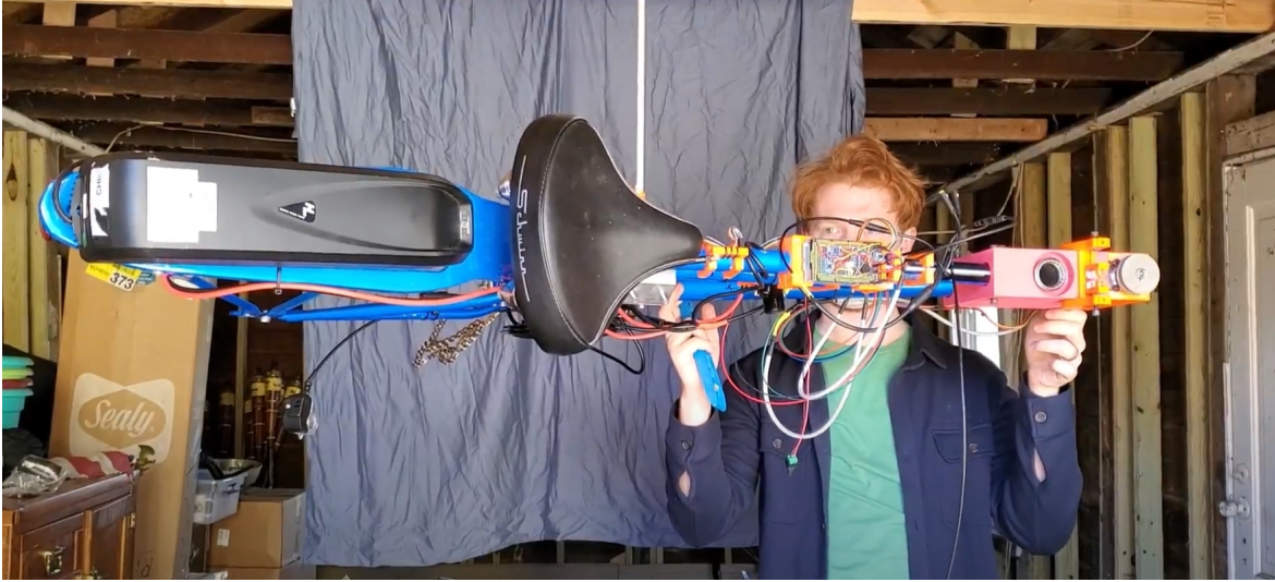
Figure 4.9: Moment of inertia testing on the back frame of the Autocycle. A perturbation is applied in the axis of rotation of the hanging metal rod, and the torsional period of rotation is measured using film playback to determine the moment of inertia around this axis.
