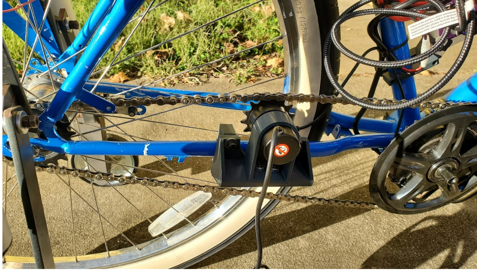
Figure 4.15: Using a 3D printed mount, the rotary encoder is connected in line with the Autocycle's chain to report accurate velocity readings.
