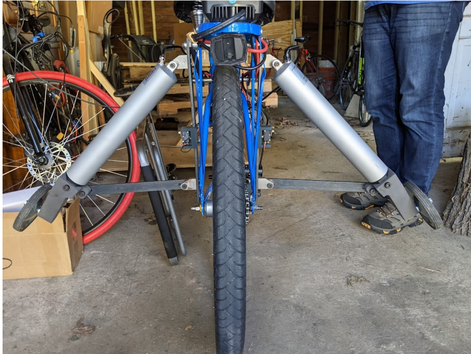
Figure 4.13: The revised ZSS geometry resulted in higher clearance provided by the wheels, allowing the Autocycle to tilt at least 30 degrees without contacting the ground.
