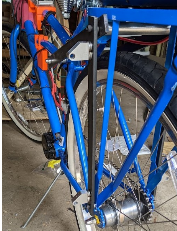
Figure 3.10: 1080 steel bars were selected for the ZSS linkage structure. The frame attaches to the chassis near the aft wheel axle, below the seat, and a threaded aluminum crossbar that both sides of the ZSS would affix to.
