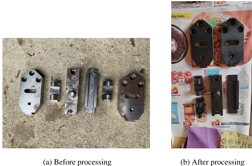
Figure 3.30: Belt tensioner components before and after de-rusting and bluing.
