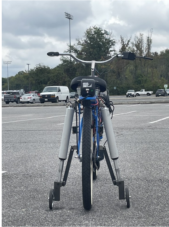
Figure 3.9: The first ZSS prototype in the "deployed" configuration. The linear actuators on either side of the bike may raise or lower the stabilizing wheels by retracting or extending, respectively.
