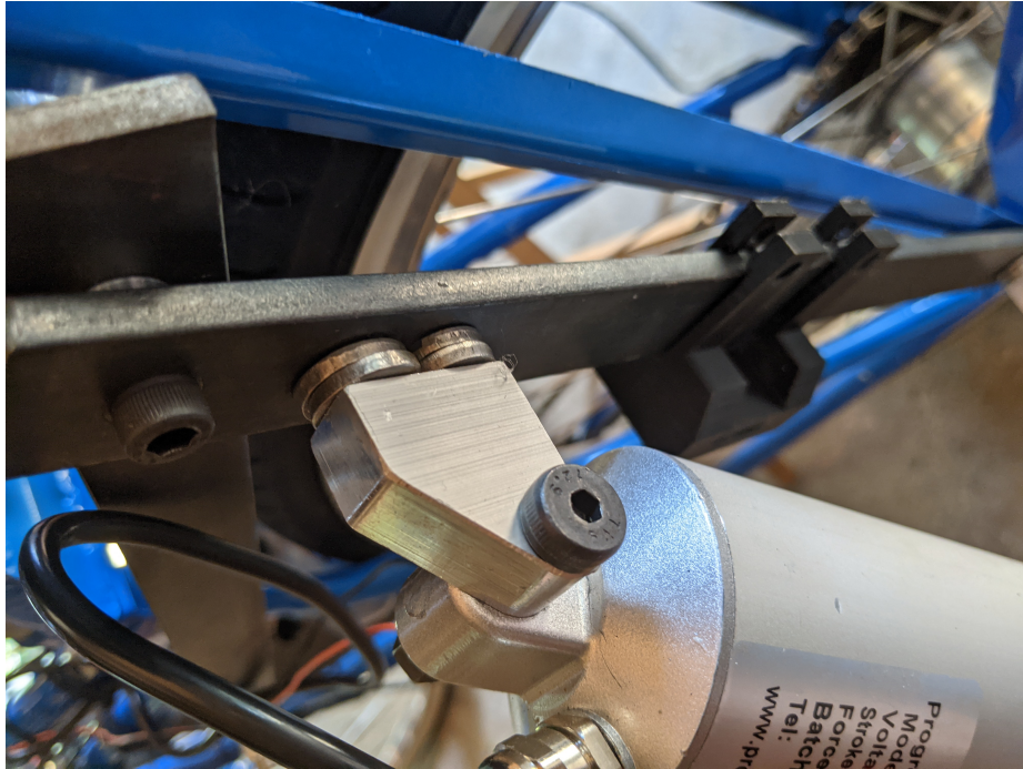
Figure 5.2: The aluminum brackets used to retain the linkage arm and linear actuator required customized spacers to keep the components of the ZSS in plane.
