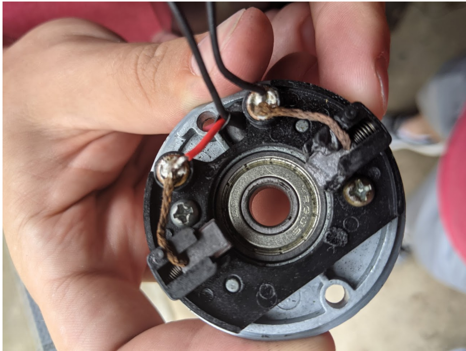
Figure 5.1: The brushed motor retained its graphite brushes inside of a plastic housing. It was a common failure for this housing to melt, and render the brush unusable.
