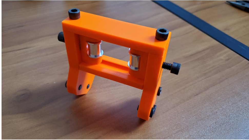
Figure 4.6: In the revised design, rollers were connected with a top bar that removed the cantilevered loading setup which previously lead to failure. This design functioned on the Autocycle until a new material was needed later on in testing.
