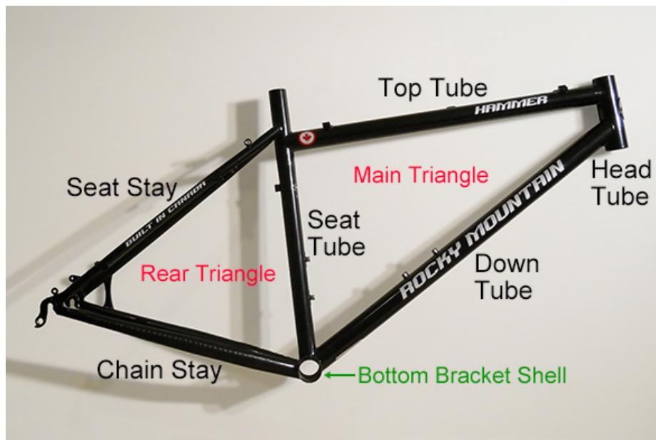
Figure 3.3: Labeled parts of bicycle frame
