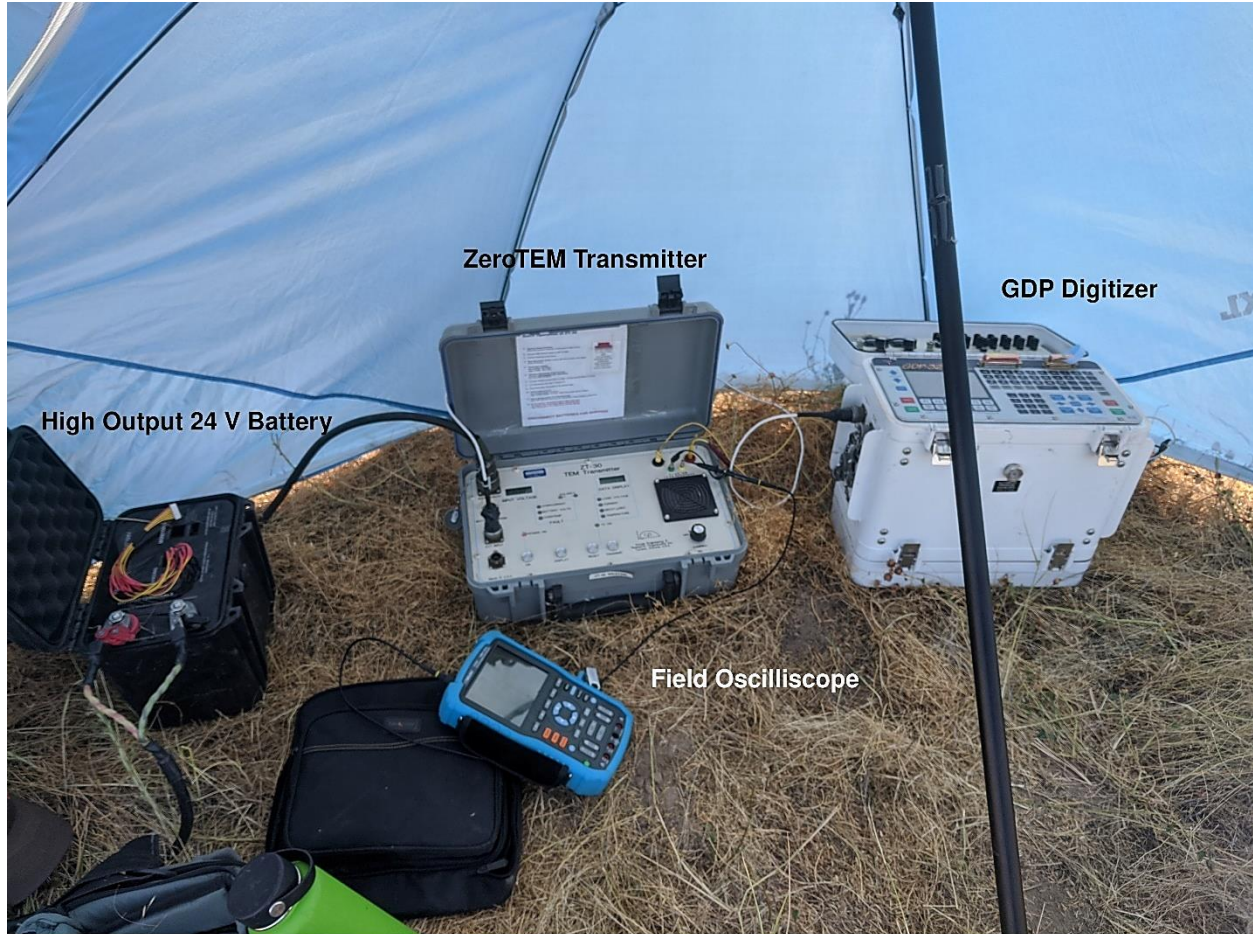
Figure 10. Field equipment set up of the transmitter and recording instrumentation under a shade structure.
