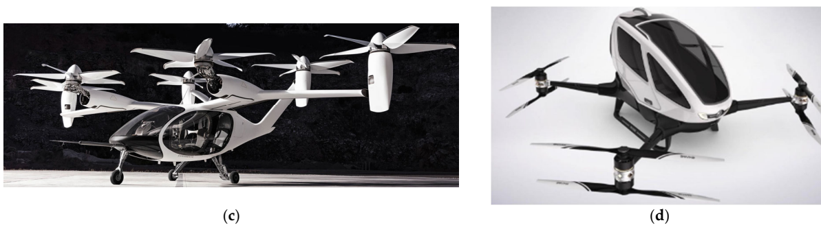
Figure 1. Different e-VTOL configurations developed from 2016: (a) Tilt-Wing (T-W) [25]; (b) Lift+Cruise (L+C) [26]; (c) Tilt-Rotor (T-R) [27]; (d) Multi-Rotor (M-R) [28].
