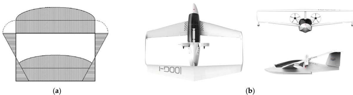
Figure 4. Example of box-wing architecture: (a) Lift distribution of the “best wing system” [62]; (b) Views of the 2-seater amphibious PrandtlPlane “IDINTOS” [64,65].
