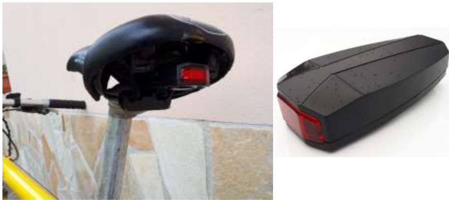
Fig. 4. The Bluetooth sensor and an example of its installation on a bike
