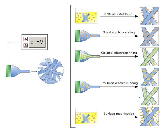
Figure 4. Fabrication techniques of biomolecule-loaded electrospun fibers.
