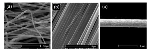
**Figure 3.** Different arrangements of fiber deposits obtained through electrospinning: (**a**) random, (**b**) oriented, and (**c**) yarn. Unpublished original pictures by the authors. All these structures are obtained through the electrospinning of PLA (original images from the authors).
