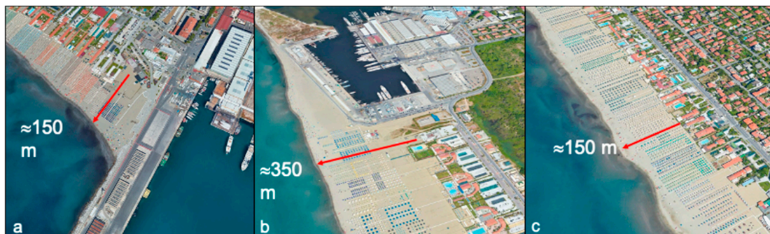
Figure 10. Aerial views of three hotspots along the Northern Tuscany littoral cell with the indication of beach width. (a) updrift beach at the Port of Marina di Carrara; (b) updrift beach at the Port of Viareggio; (c) the convergence area at Marina di Pietrasanta. The images were retrieved from the GoogleEarth database.
